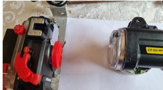
5 - Activate the shutter once – The indicator light will probably remain red. Activate the camera shutter again - the strobe indicator light should now turn green. (At least it did for me). Activate the shutter again within 3 to 5 seconds.
