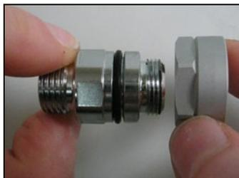
**NOTE:** There will be some slight resistance removing the two parts above due to the o-ring (11) underneath the inlet shroud (12).
