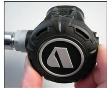
**3** Install the o-ring (11) onto the venturi lever (24). Align the venturi lever in a vertical position with the case (7) and press the lever into place. Ensure that the venturi lever rotates freely and feels secure.
