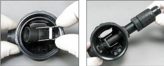
**CAUTION:** DO NOT use the lever to push the spindle body into the case as this will bend the lever.
