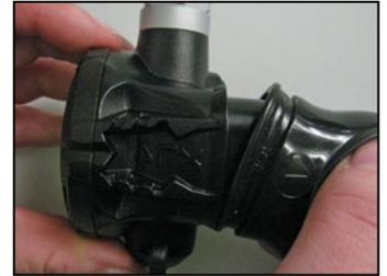
**5** To remove the clamp ring (1), place your thumb on the top of the clamp ring as shown on the first image below. Grip the rest of the clamp ring and turn counter-clockwise. Separate the purge clamp ring (1) from the purge button assembly and the case (7).
