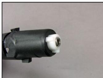
**4** Position the large fin of the spindle body (16) down. Press the end of the shuttle valve (18) to fully compress the spring (20), until it passes the triangular shaped hole in the spindle body. Insert the feet of the lever (15) one leg at a time into the gap, this retains the shuttle valve inside the spindle body.
