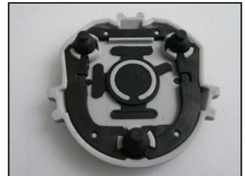
**2** Check that the tab of the venturi lever (24) has not been over stressed and that it is level with the rest of the lever.
