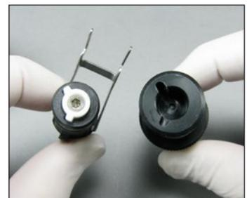
**7** Carefully insert the spindle body assembly into the case (6). Insert the tool into the venturi side of the case, carefully rotate the tool until the cutout in the tool engages with the spindle body assembly. Push the spindle body firmly into the case, ensuring that there is no gap between the two parts. Ensure that the lever (22) has a full range of movement and does not catch on the spindle body.
