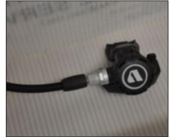
**2** Observe any bubbles arising from the submerged regulator over a one minute period. The recommended time is necessary due to slower bubble formation that occurs in smaller leaks. Bubbles indicate a leak, which requires the system to be disassembled at the source to check sealing surfaces, assembly sequence and component positioning in order to correct the problem(s).
