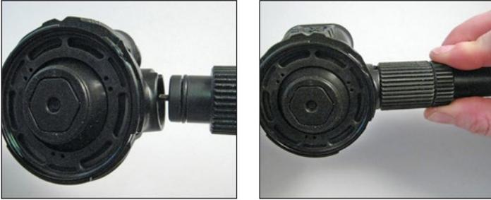
**11** Connect the first stage regulator to a calibrated test bench and pressurize the system to 3000 psi (207 bar).
