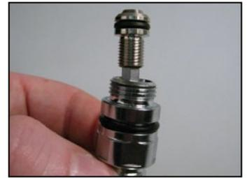
**CAUTION:** Take care when handling the seat (14). The sealing surface of the seat must be protected from damage or the regulator will leak.
