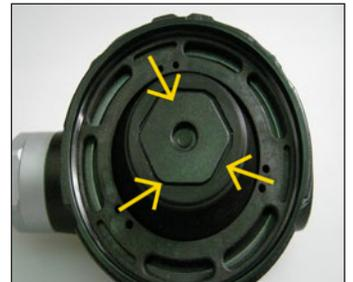
**4** Place the "GAS FLOW" side of the lever setting tool (RA911116) onto the plastic pad of the diaphragm (6). Depress the diaphragm by pushing the tool in until it stops against the case (7).
