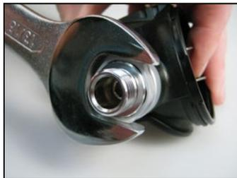
**10** The inlet shroud assembly (10/12) will remove as one. To separate, grip the regulator hose thread on the inlet fitting (10) and slide off the inlet shroud (12).
