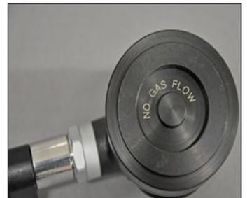
**NOTE:** The second stage "SHOULD LEAK AIR" with this test. If it does not, the lever is set too low.
