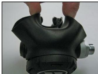
**4** Unfasten the mouthpiece clip (8) and pull the mouthpiece off the case (7).
