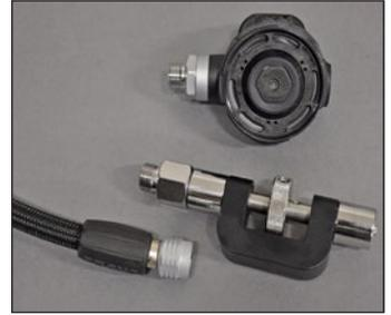
**CAUTION:** When removing the inline adjustment tool from the second stage, remember to pull the handwheel back to disengage it from the seat. Failure to perform this step can cause changes to your adjustment.
