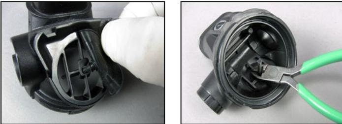
**WARNING:** Flooding may occur if the tail of the valve is not fully pulled through. Ensure that the barb has engaged on inside of case.
