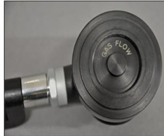
**NOTE:** The second stage **“SHOULD NOT LEAK AIR”** with this test. If it does, the lever is set too high.
