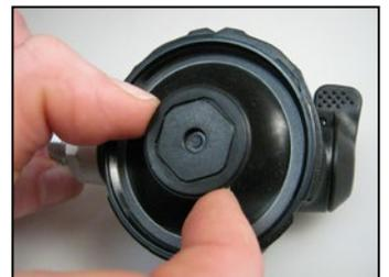
**7** Position the venturi lever (24) vertically. Using the venturi lever removal tool (RG911232), align the cutout in the tool so it will engage the tab of the venturi lever and evenly set the tool on the top of the case (7). Carefully pushing down on the tool will depress the tab of the venturi lever allowing you to remove the venturi lever from the case.
