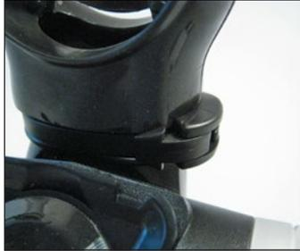
**WARNING:** Ensure that the mouthpiece is properly secured on the outlet port.
