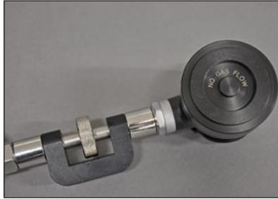
**6** Place the **“NO GAS FLOW”** side of the lever setting tool ( RA911116) onto the plastic pad of the diaphragm (6). Depress the diaphragm by pushing the tool in until it stops against the case (7).
