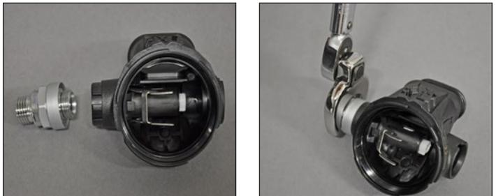
**13** While holding the case (7) at eye level, use a 5mm hex key to turn the seat (14) clockwise until the lever (15) drops just below the rim of the case. Check by gently flicking the lever, it should bounce and have free movement. The lever should return to its set position, if it sticks then the lever is not square, fitted incorrectly or it is bent.
