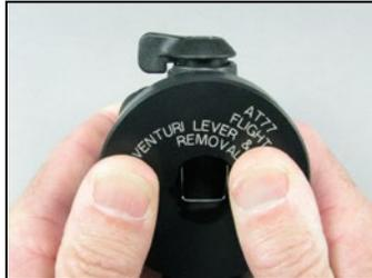
**CAUTION:** Take care not to damage or distort the venturi tab when removing the venturi lever (24). DO NOT depress the tab of the venturi lever too far, as this will result in permanent deformation.
