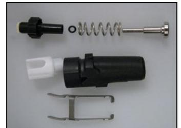
**15** Using your fingernail, remove the MP seat (17) from the shuttle valve (18).
