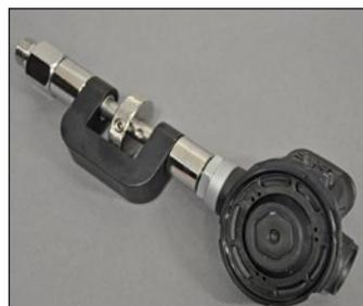
**2** Confirm the male end of the MP hose is connected to a properly adjusted first stage regulator. Thread the swivel end of the hose to the other end of the inline tool. Finally, attach the first stage to a calibrated test bench or cylinder and slowly pressurize the first stage to 3,000 psi (207 bar).
