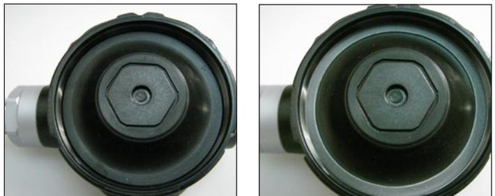
**CAUTION:** Ensure that the diaphragm (6) and friction ring (5) are seated correctly and are not creased.
