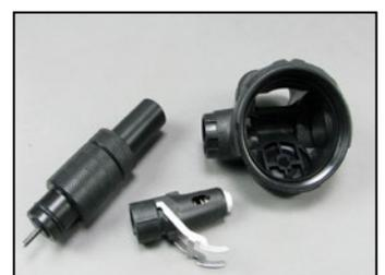
**14** To remove the lever (15) from the spindle body (16), press a finger into the end of the spindle body to compress the spring (20). Carefully pull one of the legs of the lever out of the spindle body and then ease the second leg out. Remove the shuttle valve assembly from the spindle body. Separate the components of the shuttle valve assembly.
