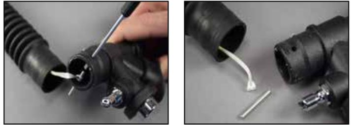
**4** Using side cutters, snip the upper clamp (11) at the buckle. Carefully remove the ribbed hose (12) from the elbow (4).
