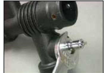
**19** Replace the retainer loop (3) if removed during disassembly. Install the retaining pin (5) halfway into the body.
