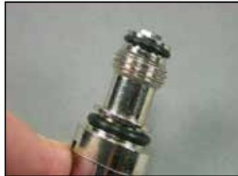
**16** Insert the valve module (16) into the body. Tighten down using the Apeks Inflator Tool (pn 15762) until snug.
