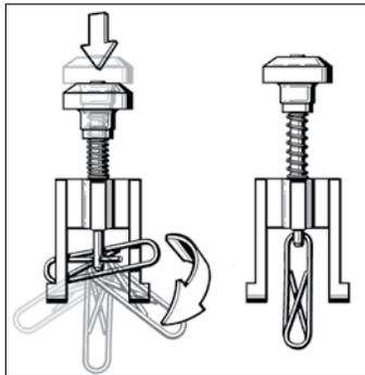
**8** With the Spectra cord (13) doubled up, make sure the knot is in the center of the cord. Take one end of the cord and thread it through the double-looped end of the hook (10). Take the other end of the cord and bring it through the loop in the cord creating a Larks Head knot. Pull the knot snug.
