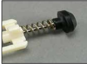
**7** Compress the poppet spring (8) and install the inflator cable hook (10) onto the poppet stem (7). The hook should be held at the single-wire end.
