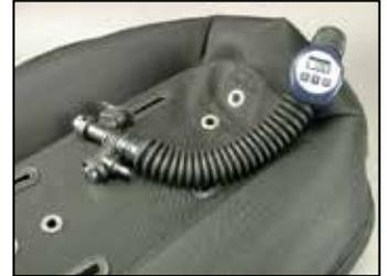
**12** If the air cell has begun to deflate within one hour, fully inflate the air cell once again and hold the entire unit completely submerged in fresh water for at least one minute to determine the source of the air loss. Carefully observe the inflator for any signs of bubble formation indicating a leak, especially around the inflator button, ribbed hose & manifold connection. If a leak is found, refer to **Table 1: Troubleshooting Guide**.
