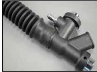
**22** Take note of raised edge on body. Lightly fasten two clamps (11) over the ribbed hose (12), one below and one above the raised edge of the body. Position both buckles to the side. Pull tight by hand. Using side cutters, trim the excess strap.
