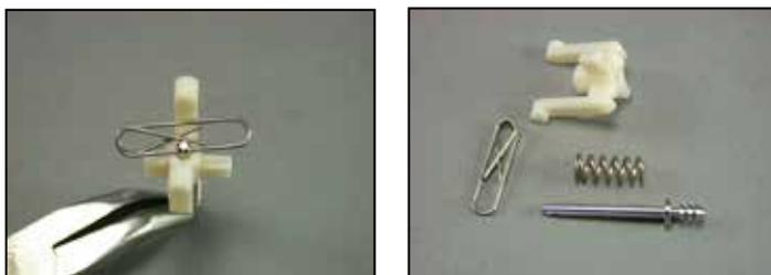
**11** Using the Apeks Inflator Tool (pn 15762), remove the inflation valve module (16) from the inflator body.
