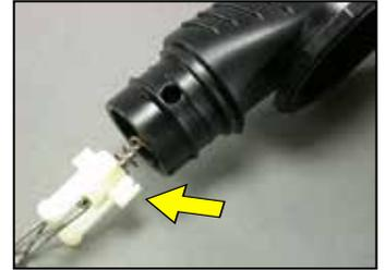
**10** Squeeze poppet guide (9) feet together and push into elbow (4). Confirm poppet guide is locked into place and poppet guide feet are seated flush with the elbow on both sides.
