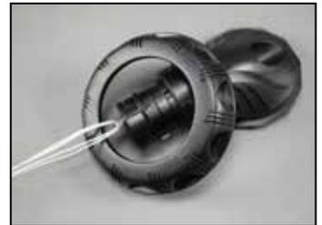
**12** Insert the Spectra cord (13) through the ribbed hose (12). If needed, use a large paperclip as a weight to get the cord to slide through the ribbed hose.
