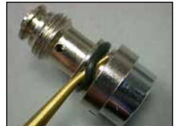
**13** Using a 1/2" open end wrench, remove the quick disconnect fitting (14) from the body. Remove the o-ring (15).
