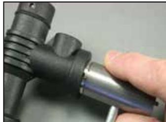
**17** Install new o-ring (15) onto quick disconnect fitting (14).
