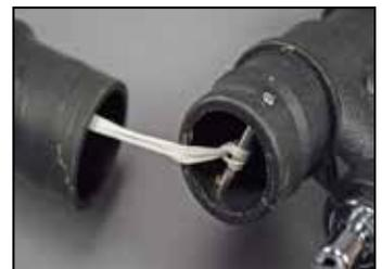
**21** Brush a thin layer of Gaseqinch onto the body. Slide the ribbed hose (12) onto the body up to the edge. Align the ribbed hose and body so there is no twist.
