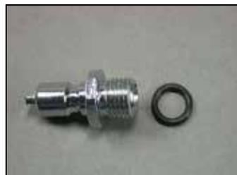
**18** By hand, carefully thread the QD fitting (14) into the body. Using a 1/2 inch open end wrench, tighten down the QD fitting until snug.
