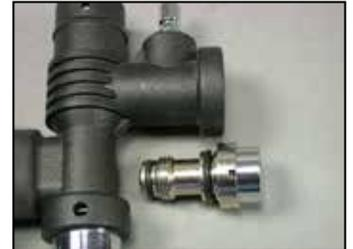
**CAUTION:** Do not attempt to disassemble the valve module. The valve module is assembled with permanent Loctite and can not be disassembled. No internal service parts are available for the module. Attempting to disassemble the valve module will cause permanent damage to the module requiring replacement of the module assembly.
