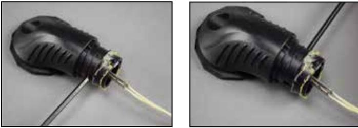
**8** Pull down on the Spectra cord (13) to remove the poppet guide assembly (6-10) from the elbow (4). Once the poppet guide assembly is out, remove the poppet dump valve (6).
