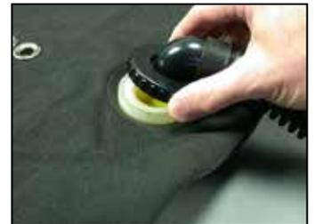
**4** Install a MP inflator hose to a properly adjusted first stage. Attach the first stage to a cylinder filled to 3000 psi (206 bar). Attach the hose to the quick disconnect fitting on the inflator.
