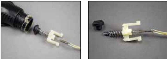
**9** Remove the Spectra cord (13) from the inflator cable hook (10).
