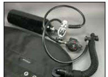
**6** Depress the inflator button several times to ensure that airflow is unobstructed, DO NOT completely fill the air cell. After releasing the button, listen carefully to ensure that the airflow has completely stopped. If airflow continues, de-pressurize and refer to **Table 1: Troubleshooting Guide**.
