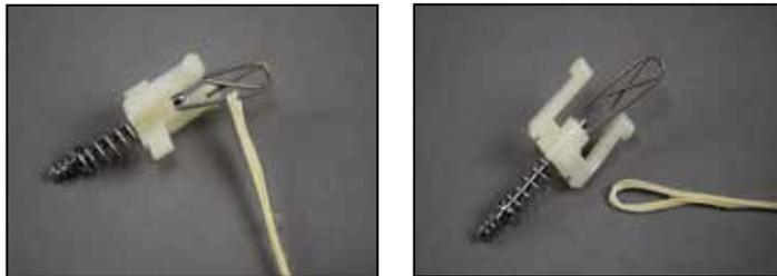
**10** Use needle nose pliers to gently grip the end of the poppet stem (7). Separate the inflator cable hook (10), poppet stem, pull dump spring (8) and poppet guide (9).
