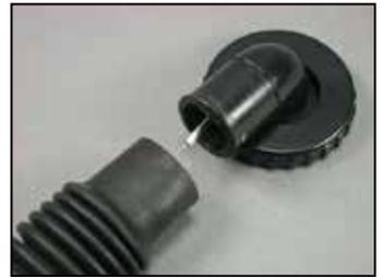
**4** Brush a thin layer of Gasgacinch onto the elbow (4). Slide the ribbed hose (12) onto the elbow up to the line. Align the ribbed hose so the flat side is against your body.
