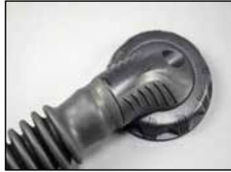
**14** Lightly fasten a clamp (11) over the ribbed hose (12). Position the buckle of the clamp to the side. Pull tight by hand. Using side cutters, trim the excess strap.
