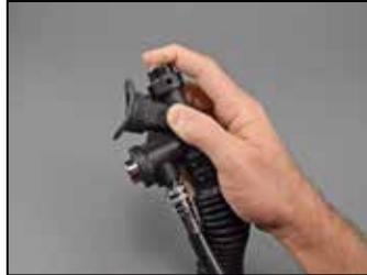
**8** Hold the inflator button depressed to fully inflate the air cell until an over-pressure relief valve opens to release the excess pressure.
