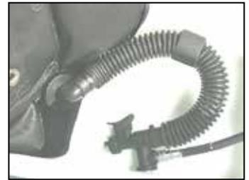
**11** If leaks were not detected, confirm the air cell is fully inflated. Disconnect the MP inflator hose from the quick disconnect fitting. Set a timer for one hour to ensure there are no leaks. If air loss occurs, depressurize and refer to **Table 1: Troubleshooting Guide**.
