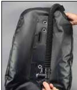
**10** With the air cell fully inflated, listen for any leaks. Submerge the entire inflator assembly in fresh water and check for any bubbles. If a leak is found, depressurize and refer to **Table 1: Troubleshooting Guide**.
