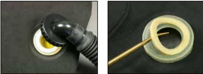
**2** Using side cutters, snip the two lower clamps (11) at the buckle. Carefully remove the ribbed hose (12) off the inflator body.
