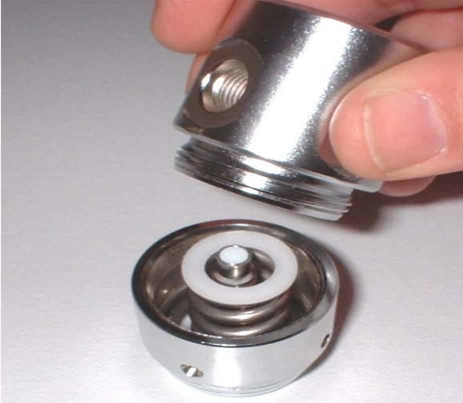
Tighten the endcap until it's secure against the first stage body. Torque to 12 ft/lbs.
