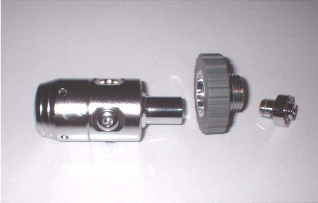
With the filter retainer removed, the conical filter should drop out of the DIN connector.
