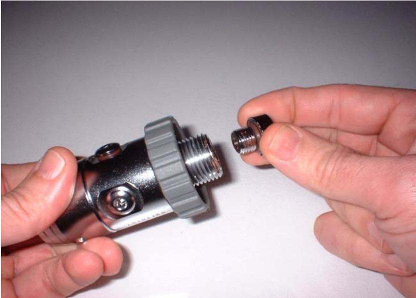
Use an allen wrench to tighten the filter retainer to the DIN connector body.
