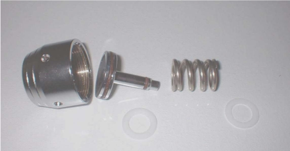
Use an allen wrench to remove the filter retainer from the DIN connector assembly.
