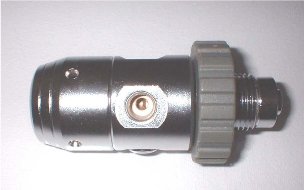
Secure the first stage (end cap up) in a padded vise being careful not to scratch or damage the chrome finish. You can also thread an expended CO2 cartridge into a low pressure port to provide a work handle.
