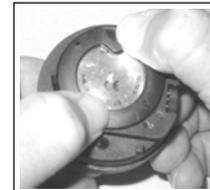
Fig. 69 - ENGAGING the RETAINING RING TABS
