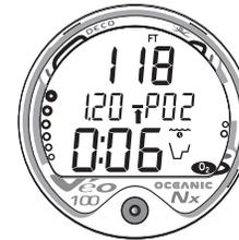
Fig. 47 - HIGH PO<sub>2</sub> WARNING
