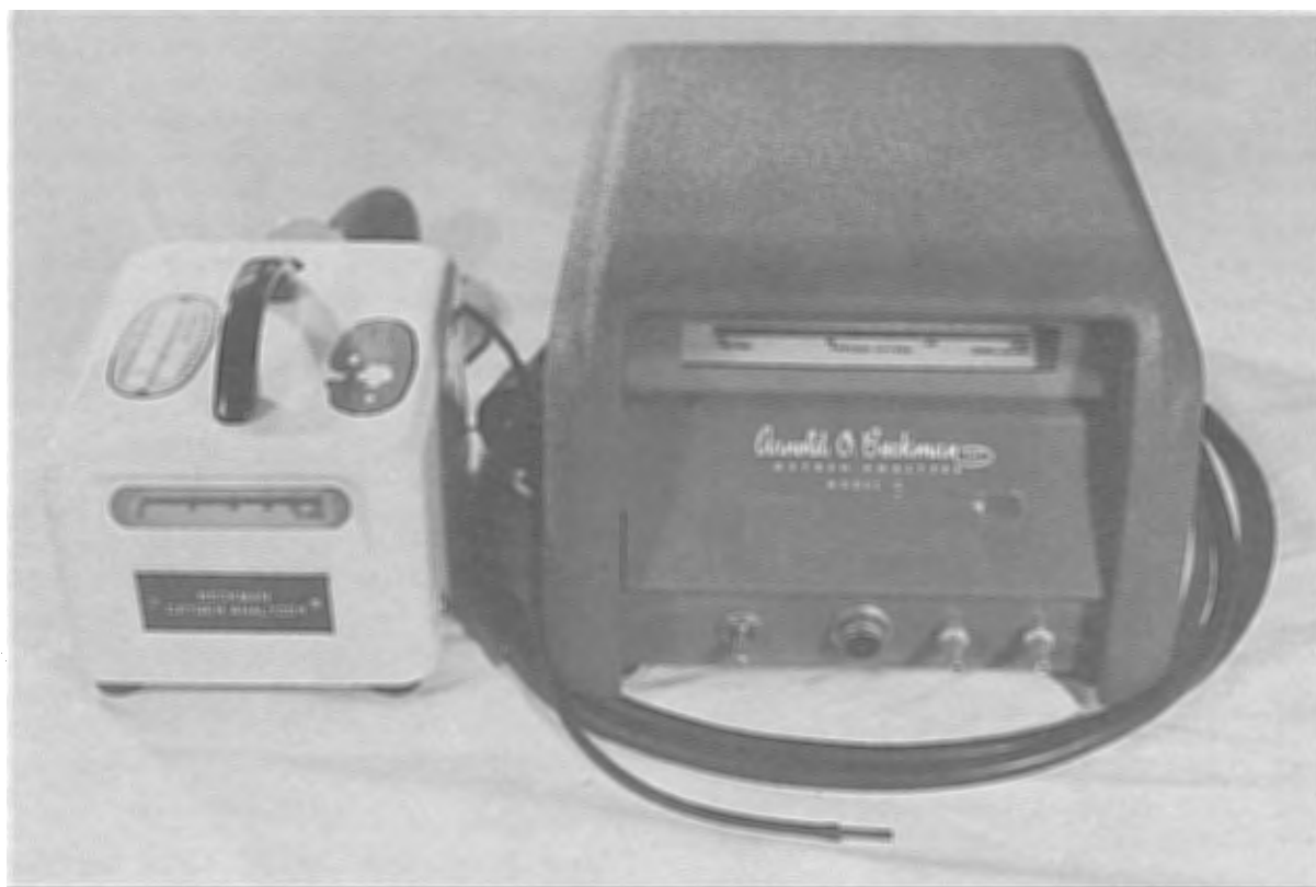
FIGURE 1-58.—Beckman oxygen analyzers. Left, Model D; right, Model C.
