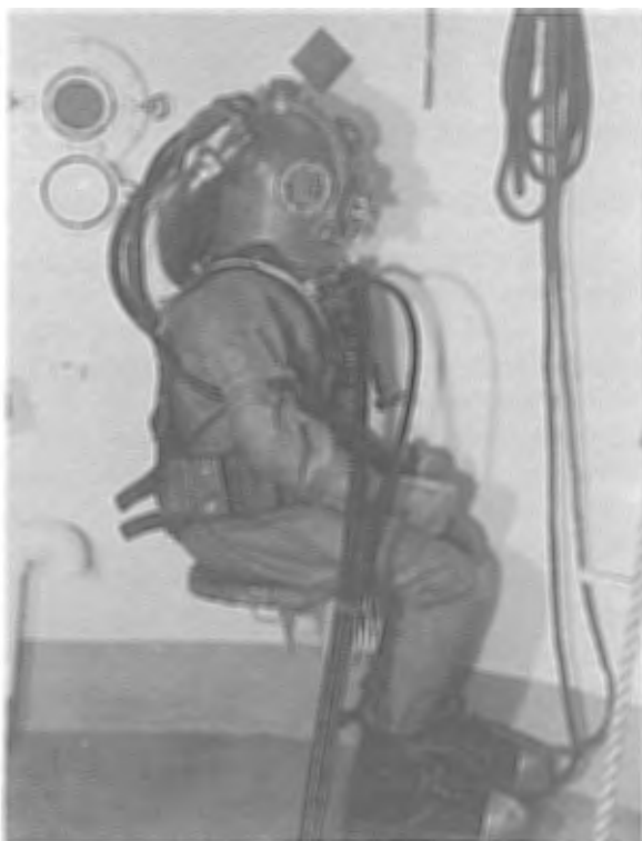
FIGURE 1-9.—Surface-supplied apparatus: helium-oxygen equipment.
