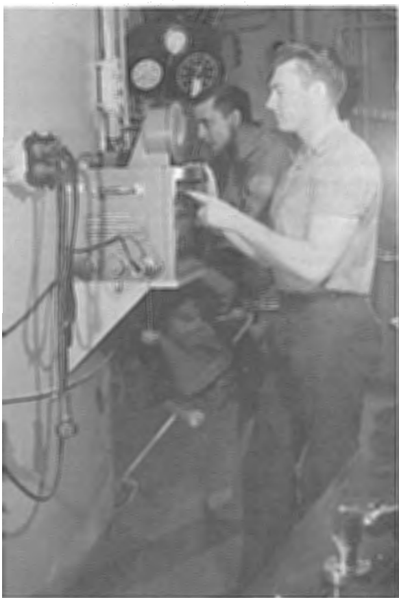
FIGURE 1-3.—Pressure tank, Experimental Diving Unit. The two wet-pressure tanks in the Deep Sea Diving School are used for training in deep diving; those in the Experimental Diving Unit are employed in the testing of decompression tables and for experimental dives.
