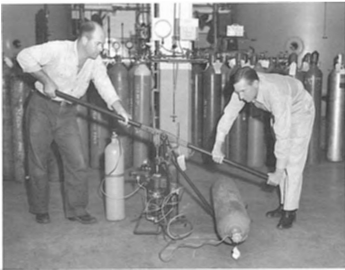
FIGURE 1-53.—MSA booster pump.
