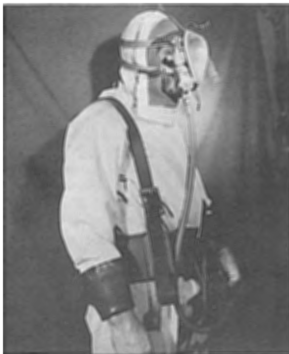
FIGURES 1-8.—Surface-supplied apparatus: lightweight diving outfit.
