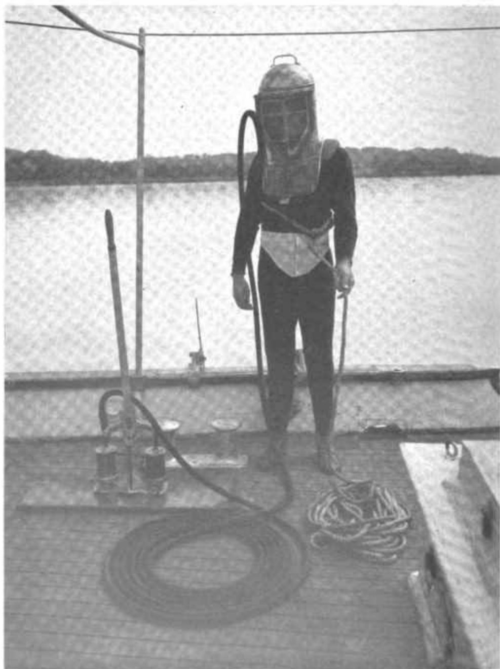
PLATE 76.—Shallow water diving apparatus—Miller-Dunn type.
