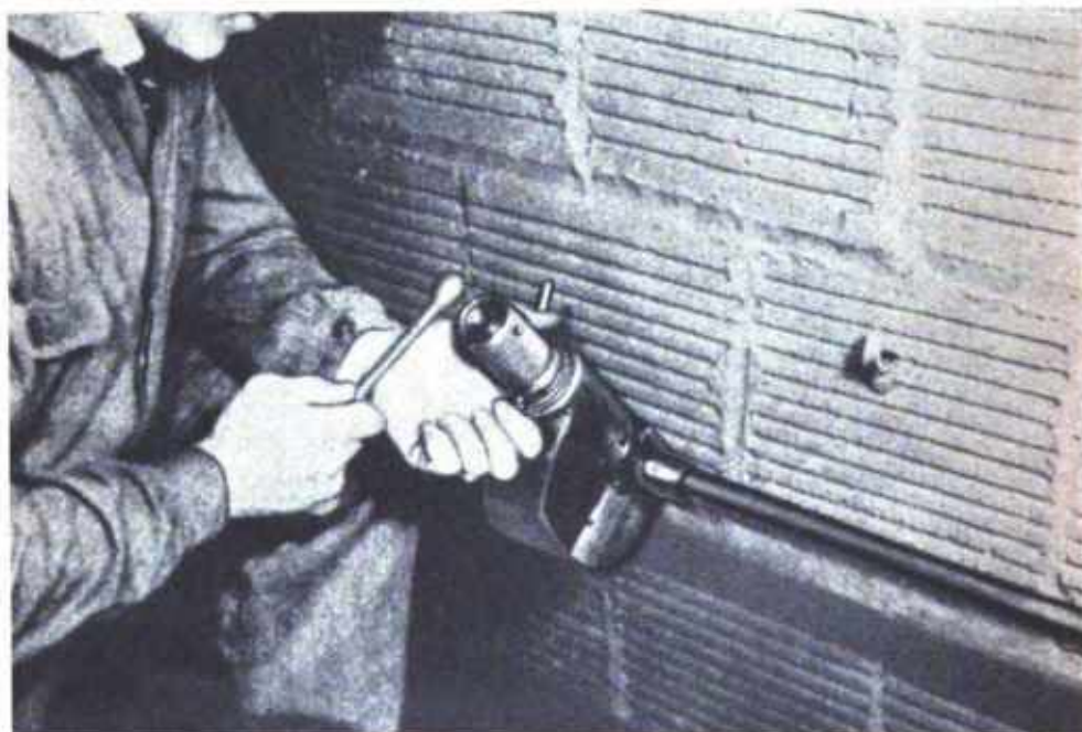
PLATE 104.—Velocity power pipe bonding press.
