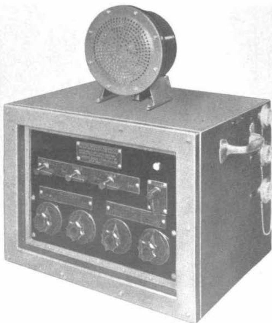
PLATE 73-A.—Amplifier and tender's reproducer front and right side.
