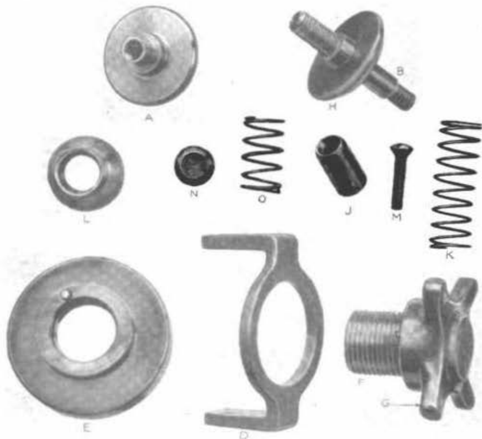
PLATE 27-A.—Helmet, air-regulating escape valve, disassembled.
