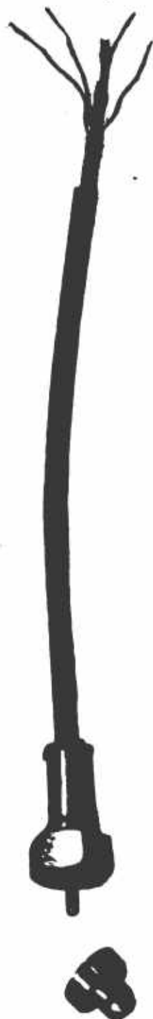
PLATE 14.—Standard rubber-covered combination telephone and life-line cable.
