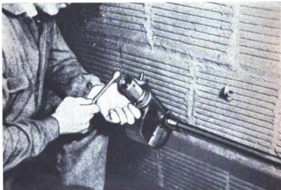
PLATE 104.—Velocity power pipe bonding press.
