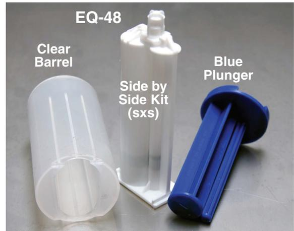
EQ-49 is an adapter that can be used to dispense material from a side by side (sxs) kit, aka dual cartridge, in conjunction with a standard caulking gun. The EQ-49 adapter contains 2 parts: clear barrel and blue dual cartridge plunger. EQ-48 is similar to the EQ-49 but uses a 10:1 two part mix ratio (note smaller cylinder on right).
