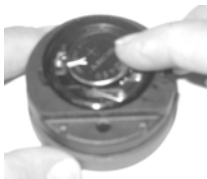
Fig. 64 -INSERTING BATTERY
