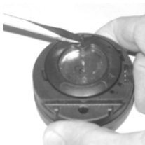
Fig. 62 - RING REMOVAL
