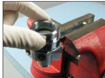
**11** Using torque wrench with the spring retainer socket (PN 122152), torque the spring retainer (6) clockwise to 18 ft-lbs (25.4 Nm)
