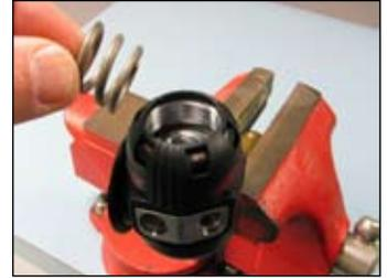
**8** Carefully lift the protector (1) using a small bladed screwdriver.
