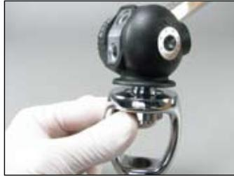
**CAUTION:** Preliminary installation of the inlet fitting requires the filter/o-ring side be facing up; keeping the filter/o-ring from dislodging and becoming damaged. Damage to the filter or o-ring can result in a HP leak.
