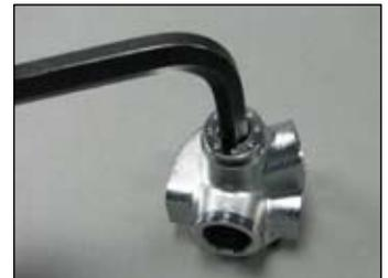
**7** Install the vise mount tool (PN 5116230) into an MP port on the body (10). Position the body in a vise so that the HP side is facing up. Using a torque wrench and an 8mm hex key adapter, torque the HP plug (18) clockwise to 45 in-lbs (4.9 Nm).
