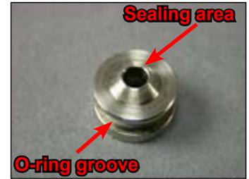
**CAUTION:** Care must be taken not to scratch the sealing surfaces of the crown orifice or a HP leak could result. Use brass or plastic o-ring tools only.
