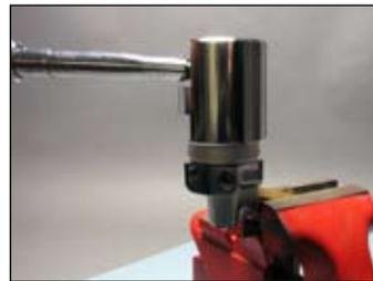
**12** Press the protective cover (1) onto the spring retainer (6).
