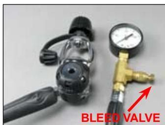
**WARNING:** Be certain not to install a MP hose into the HP port via an adapter. Doing so may cause the hose to rupture when pressurized, and could result in serious personal injury.
