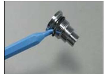
**18** Using an o-ring tool, carefully remove the o-ring (15) and the back-up ring (16) from the balancing chamber inside the HP plug (18).
