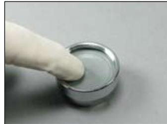
**10** Install the spring retainer (6) onto the body (10). Turn the spring retainer clockwise by hand until snug.
