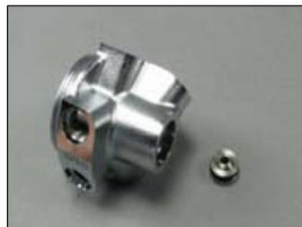
**CAUTION:** Perform this step over a padded surface. Any damage to the crown orifice can cause a HP leak to result.
