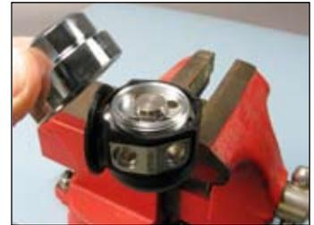
**NOTE:** Diaphragm (7) and spring pad (5) will come away with the spring retainer (6).
