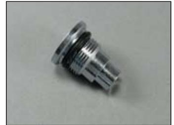
**6** Place the HP plug (18) into the body (10). Using an 8mm hex key, compress and turn the HP plug clockwise until snug.
