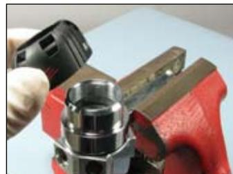
**13** Place the spring pad (5) with the raised edge facing up, into the spring retainer (6). Place the spring (4) over the raised edge of the spring pad.
