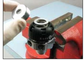
**15** Using an 8mm hex key, turn the adjustment screw (2) clockwise until it is flush with the top of the protective cover (1).
