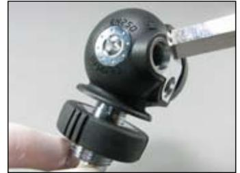
**CAUTION:** Preliminary installation of the DIN fitting requires that the filter side to be facing up; keeping the o-ring and filter from dislodging and becoming damaged. Damage to the filter or o-ring can result in a HP leak.
