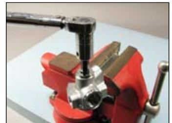
**8** Rotate the body (10) so that the MP side is facing up. Insert the pin (9) into the center hole. Place the pin support (8) onto the pin. Push down on the pin support and you should feel spring tension.
