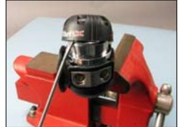
**9** Using a large, adjustable wrench turn the spring retainer (6) counter-clockwise and remove it from the body (10).
