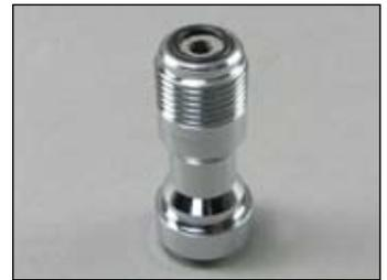
**b** Place the DIN fitting (30) through the DIN handwheel (29) being careful not to dislodge the o-ring (22) and filter (24). Hold the inlet area of the body (10) facing down, thread the DIN adapter clockwise up into the body by hand until snug.
