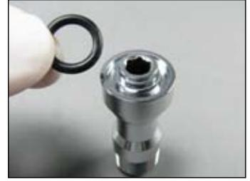
**a** Place the filter (24) into the back side of the DIN fitting (30). Install an **“UNLUBRICATED”** o-ring (22) into the groove around the filter.
