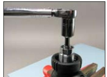
**d** Remove the first stage from the vise. Unthread the vise mount tool. Replace the protective DIN cap (32).
