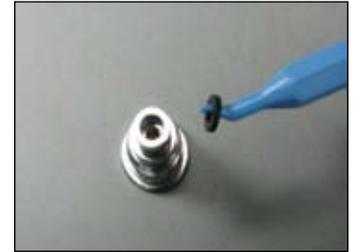
**CAUTION:** Care must be taken not to scratch the inside wall of the balance chamber or a HP leak could result. Use brass or plastic o-ring tools only.
