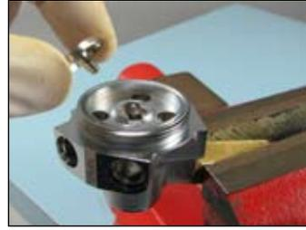
**9** Press a new diaphragm (7) into the spring retainer (6). Make sure the diaphragm is seated evenly in the spring retainer.
