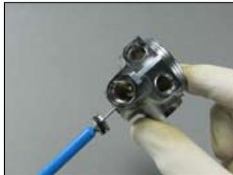
**3** Install the HP seat (13) so that the blue side rests against the sealing edge of the crown (12). Place the spring (14) over the HP seat.
