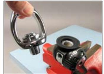
**c** Use the blunt end of the seat extraction tool (PN 109437), to push the filter (24) and the o-ring (22) out the back of the inlet fitting (25).
