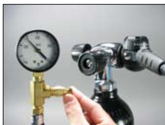
**CAUTION:** Before pressurizing the first stage, it is important to have a properly adjusted second stage attached to the first stage. This will provide a safety relief valve if the MP exceeds 145 psi (10 bar). Failure to relieve increasing MP may result in damage to the test gauge or the MP hose.
