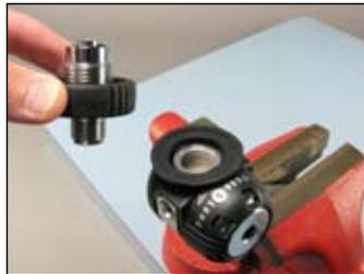
**c** Use the pointed end of the seat extraction tool (PN 109437) to carefully push the filter (24) and o-ring (22) out of the DIN fitting (30). Remove the face o-ring (31) from the DIN fitting.
