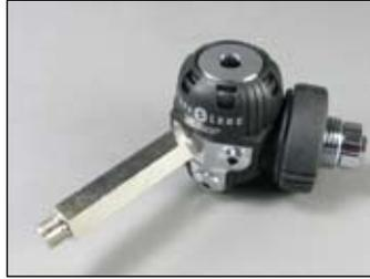
**a** Secure the vise mount tool and first stage into a bench vise with the DIN adapter facing up.
