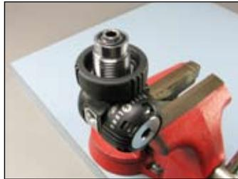
**b** Using a 6mm hex key, turn the DIN fitting (30) counter-clockwise to loosen and then lift the DIN adapter off the body (10). Separate the DIN fitting from the DIN handwheel (29).
