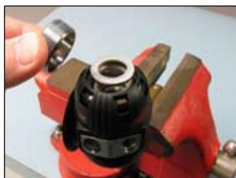
**7** Using your fingers, remove the washer (3) and the spring (4).
