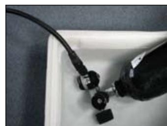
**NOTE:** Do not confuse bubbles from trapped air with a true leak. If there is an air leak, bubbles will come out in a constant stream.
