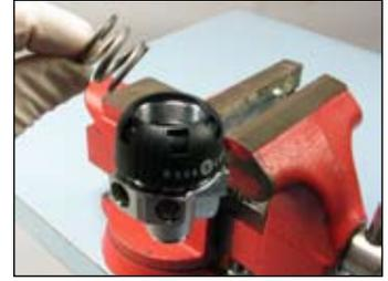
**14** Place the washer (3) directly on the top of the spring (4). Put the adjustment screw (2) over top of the washer and spring.
