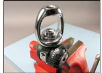
**b** Using a 8mm hex key, turn the inlet fitting (25) counter-clockwise and then lift off the yoke assembly. Remove the inlet fitting from the yoke.
