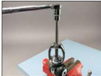
**c** Remove the first stage from the vise. Unthread the vise mount tool. Install the yoke screw (28) and the dust cap (27).
