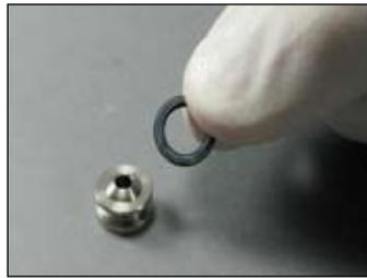
**2** Using the seat installation tool (PN 109437), place the raised area of the crown (12) against the plastic handle. Push the crown into the HP side of the body (10). Make sure the crown is seated evenly inside the body.
