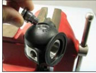
**13** Rotate the body (10) and allow the spring (14) and HP seat (13) to fall out. Remove the body from the vise.
