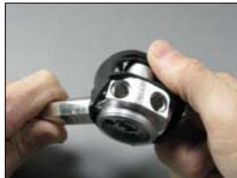
**15** Use a small dowel to carefully push the crown (12) out of the body (10).
