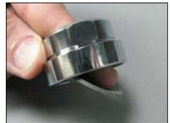
**11** Rotate the body (10) in the vise so that the HP side is facing up. This will allow the pin support (8) and the pin (9) to fall into your hand. Separate the pin and pin support.
