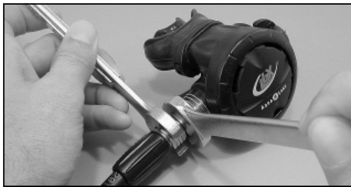
Fig. 1 – Removing the Hose
