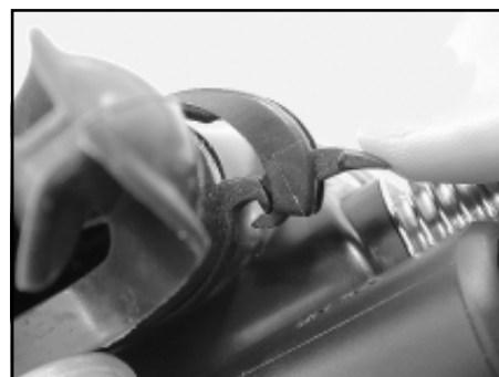
Figure 19. Installing the reusable mouthpiece clamp
