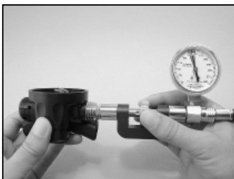
Figure 17. Using the inline adjustment tool to adjust lever height.
