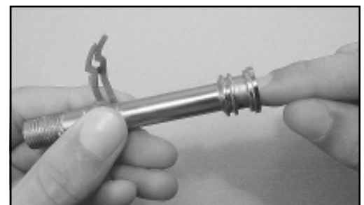
Figure 12b. Push shuttle valve all the way in
