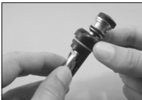
Figure 5. Remove venturi lever from valve body
