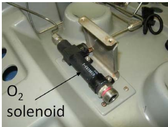
Figure 18. MK 16 solenoid.
