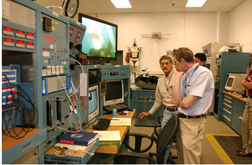
Figure 8. Control console for unmanned equipment testing.
