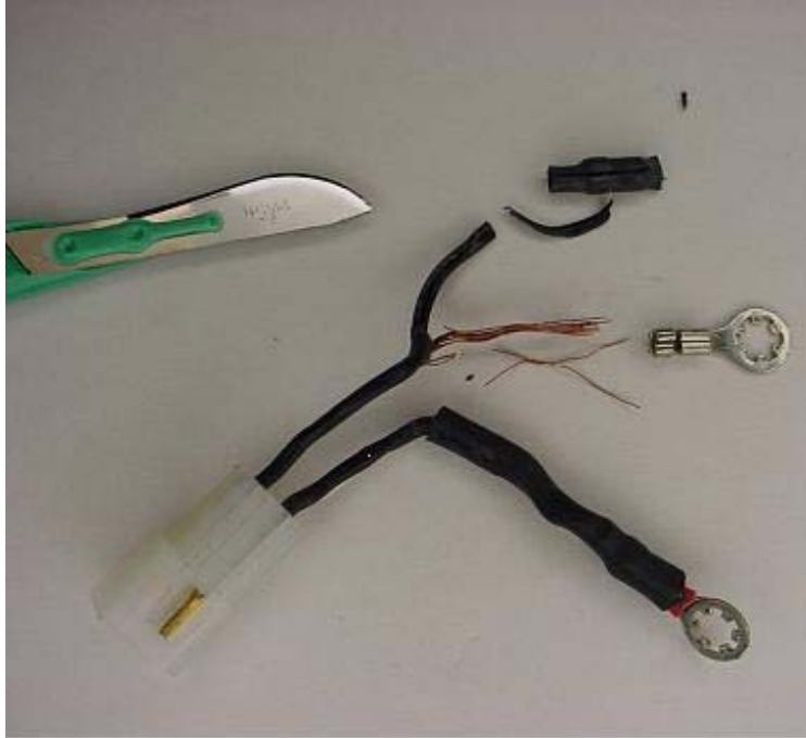
Figure 22. Connecting wires damaged by improper repair.
