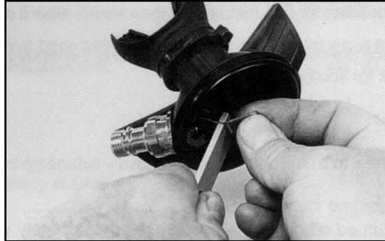
9. Holding the tool in one hand, with the tip of the lever toward the fingers, bend the lever carefully. Do not hold on to the case when making this adjustment, as this can result in the lever bending at the wrong area (near the lever support instead of at the mid-point of the lever). If necessary, bend the lever upward using the same holding method.
