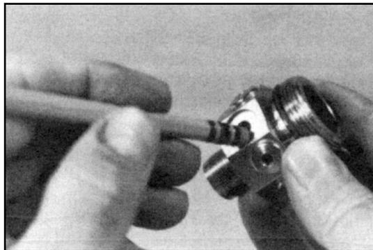
(15) Remove the large O-ring (item 20) from the Body and the large O-ring (item 22) from the Pressure Adjusting Ring.
