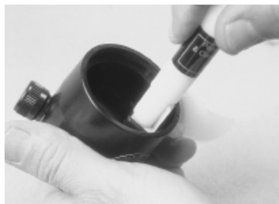
Figure 9. Poppet Housing Removal
