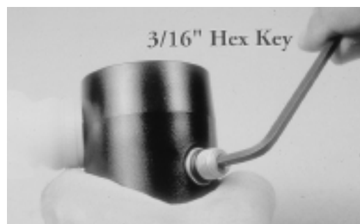
Figure 12. Check Valve Removal
