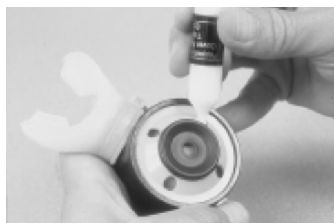
Figure 6. Purge Cover Removal, Original Regulator
