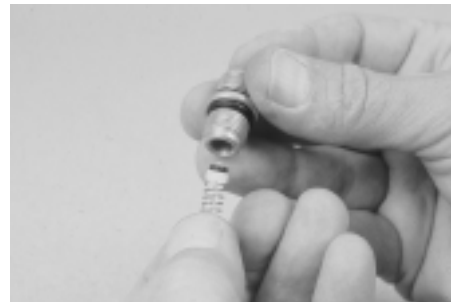
Figure 17. Check Valve Assembly
