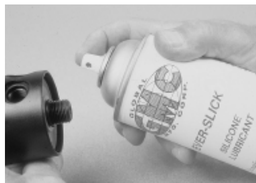
Figure 15. Thread Lubrication
