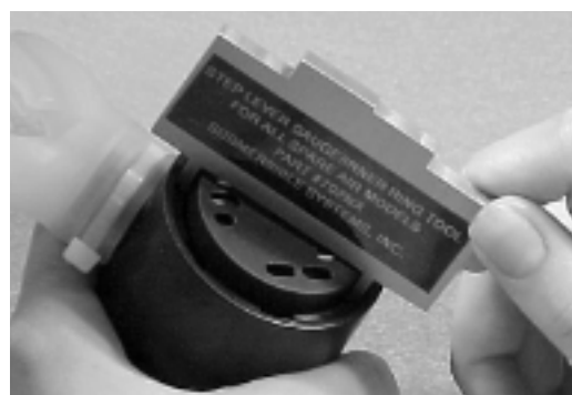
Figure 26. Inner Ring Installation, Next Generation Regulator
