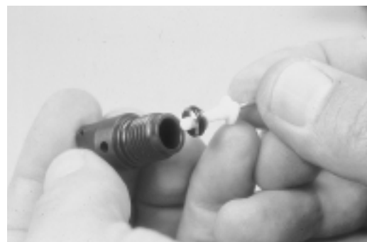
Figure 10. Poppet Seat Removal
