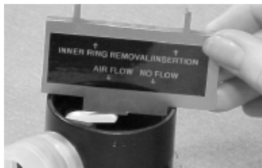
Figure 22. Checking Lever Height
