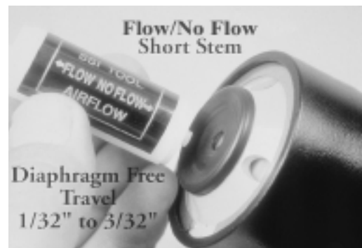
Figure 25. Final Lever Height Check with Flow/No Flow Gauge, Original Regulator
