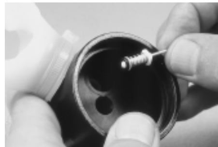
Figure 19. Poppet Assembly Installation
