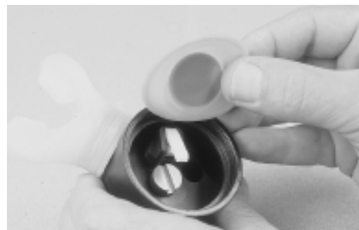
Figure 21. Back Off Poppet Housing
