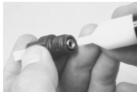
Figure 20. Poppet Seat Installation
