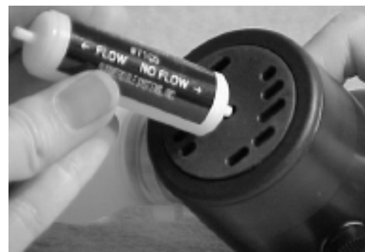
Figure 27. Final Lever Height Check with Flow/No Flow Gauge, Next Generation Regulator
