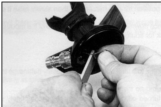
Holding the tool in one hand, with the tip of the lever toward the fingers, bend the lever carefully. Do not hold on to the case when making this adjustment, as this can result in the lever bending at the wrong area (near the lever support instead of at the mid-point of the lever). If necessary, bend the lever upward using the same holding method.
