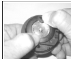
Fig. 75 - Retaining Ring Tabs
