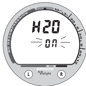
Fig. 21 - Set Wet Activation
