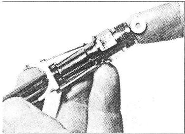
10. Place a second teflon friction washer (#13) into the demand valve sleeve (#7). (sensitivity knob end)
