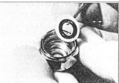
7. Remove delrin washer (#14) and small O ring (#24) from gland nut (#10).
