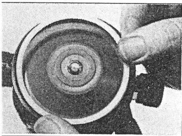
26. Place nylon friction washer (#31) over the diaphragm. (#33)
