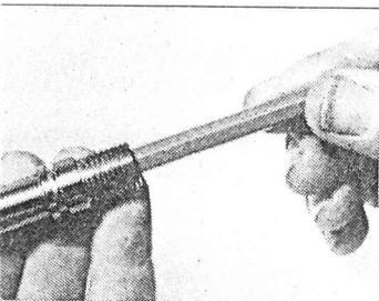
6. Install a new LP seat (#18), large end first, onto piston assembly (#8). The rubber seat should sit flat with no air trapped between the seat and the piston.
