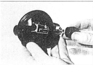
5. Undo retaining screw (#21) and remove the sensitivity knob (#5).
