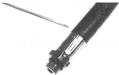
Remove LP hose from 1st stage and inspect both ends for damage, particularly near the swage fittings.
