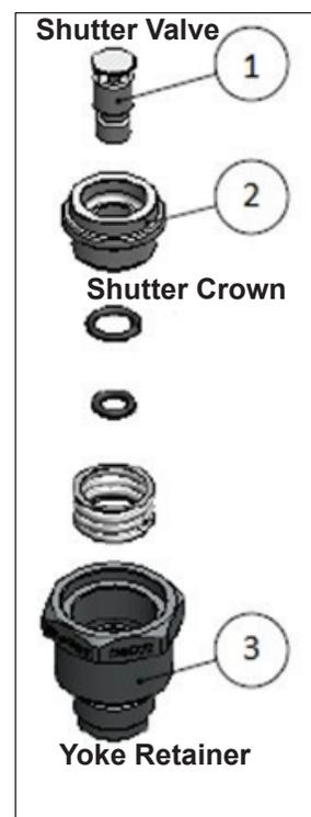
**CORRECTIVE ACTION:** If you find a gap in the Shutter Crown then you will need to remove the Yoke Retainer (3) from the regulator body and re-torque the Shutter Valve (1) to 27 in-lbs (3 Nm) following the instructions in the maintenance manual.
