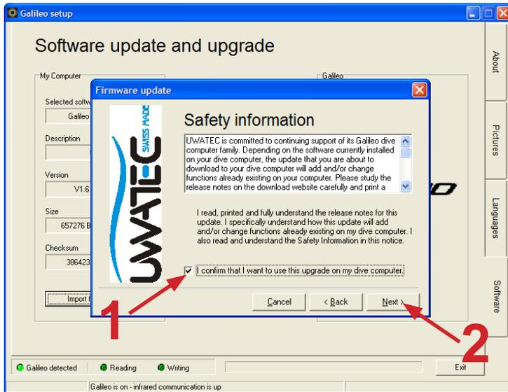
SmartTRAK now prompts you with two more messages, you must press **Next** then **Continue** to finally begin the process of uploading the new firmware on Galileo. Observe the progress bars on the screen of Galileo.
