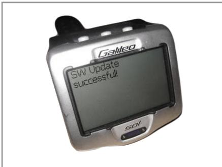
At this point push the right button for one second. This will turn off the display. Galileo is now ready for use with the new software.
