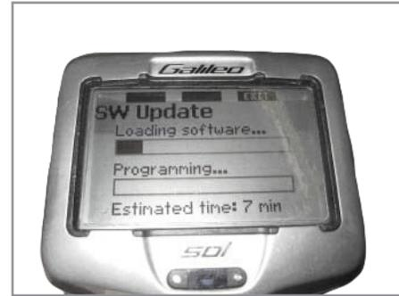
**ERROR MESSAGE:** If you get an error message at the end of the update process, unscrew the battery cap until the message goes away, then retighten the battery cap.
