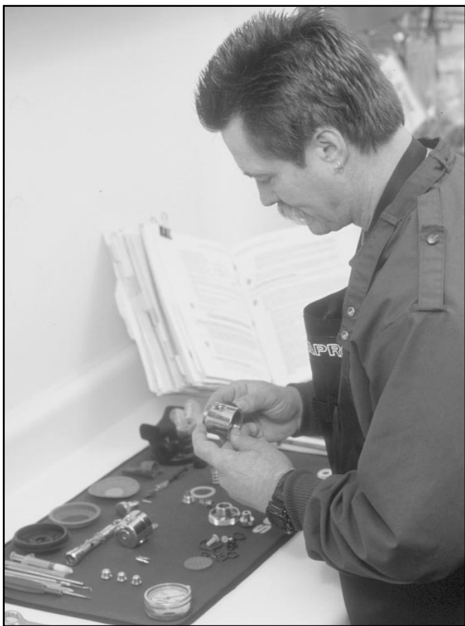
FIGURE 15.10 Preparation of Regulator Parts for Oxygen Service
