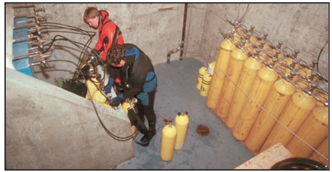
FIGURE 5.29 Fill Station
