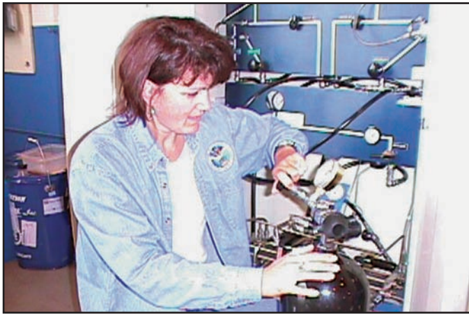
FIGURE 5.28 Air Fill Control Panel With Fill Hoses
