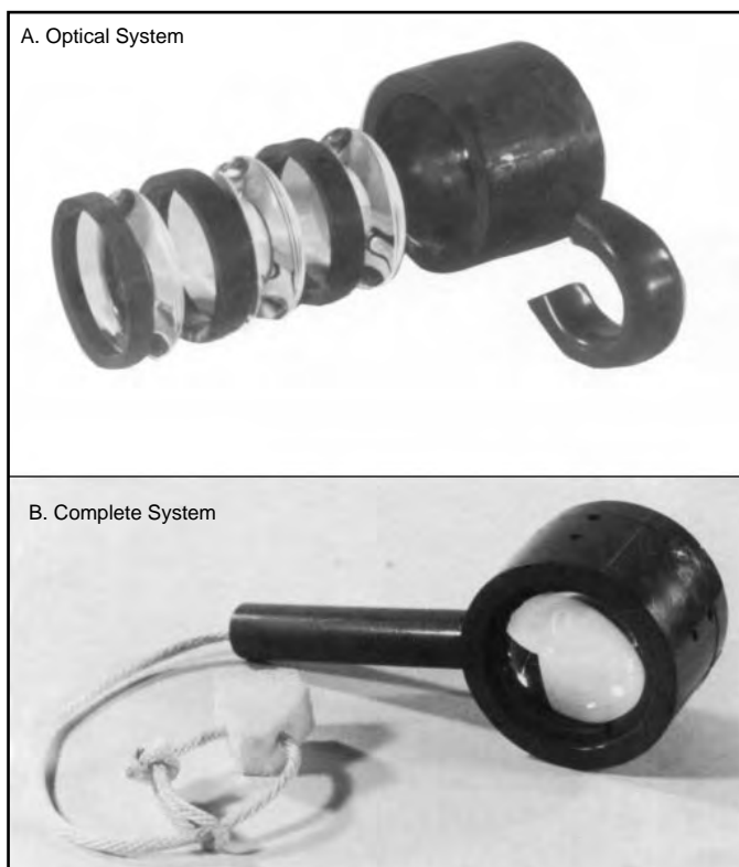
FIGURE 9.7 Underwater Magnification System
