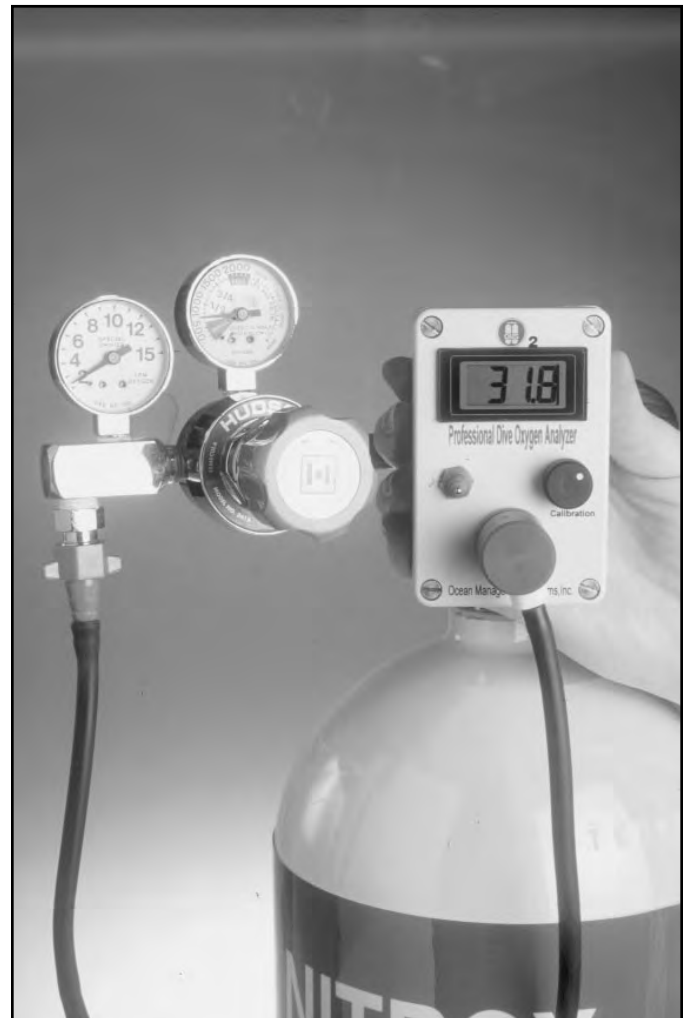
FIGURE 15.20 Oxygen Analyzer Analyzing a Nitrox Cylinder
