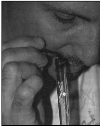
FIGURE 5.24 Internal Inspection of a Scuba Cylinder
