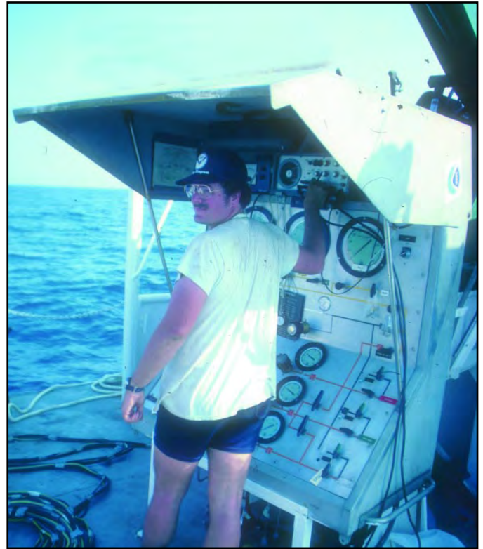
FIGURE 11.22 Diver/Open-Bottom Bell System Control Panel
