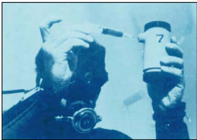
FIGURE 9.37 Custom Dissolved Oxygen Water Sampler
