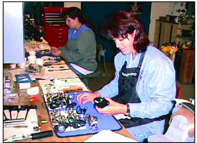
FIGURE 5.20 NOAA Technician Inspecting and Repairing Regulators
