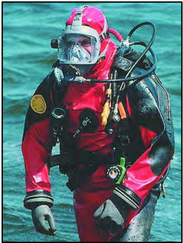
FIGURE 5.7 Heavy Duty Suit Made of Vulcanized Rubber
