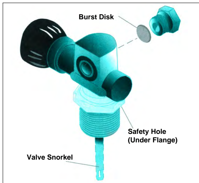
FIGURE 5.26 Cylinder Valve Safety Features
