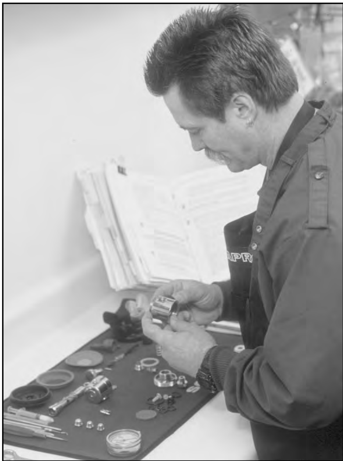
FIGURE 15.10 Preparation of Regulator Parts for Oxygen Service
