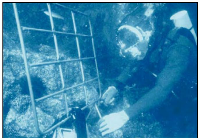
FIGURE 9.15 Electroshock grid
