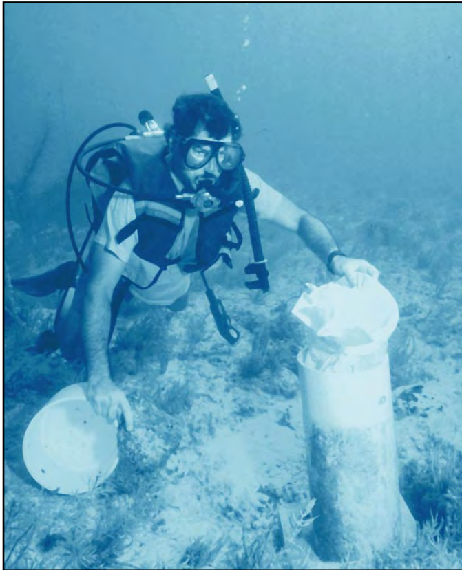
FIGURE 9.33 Deploying an Instrument Inside PVC Housing
