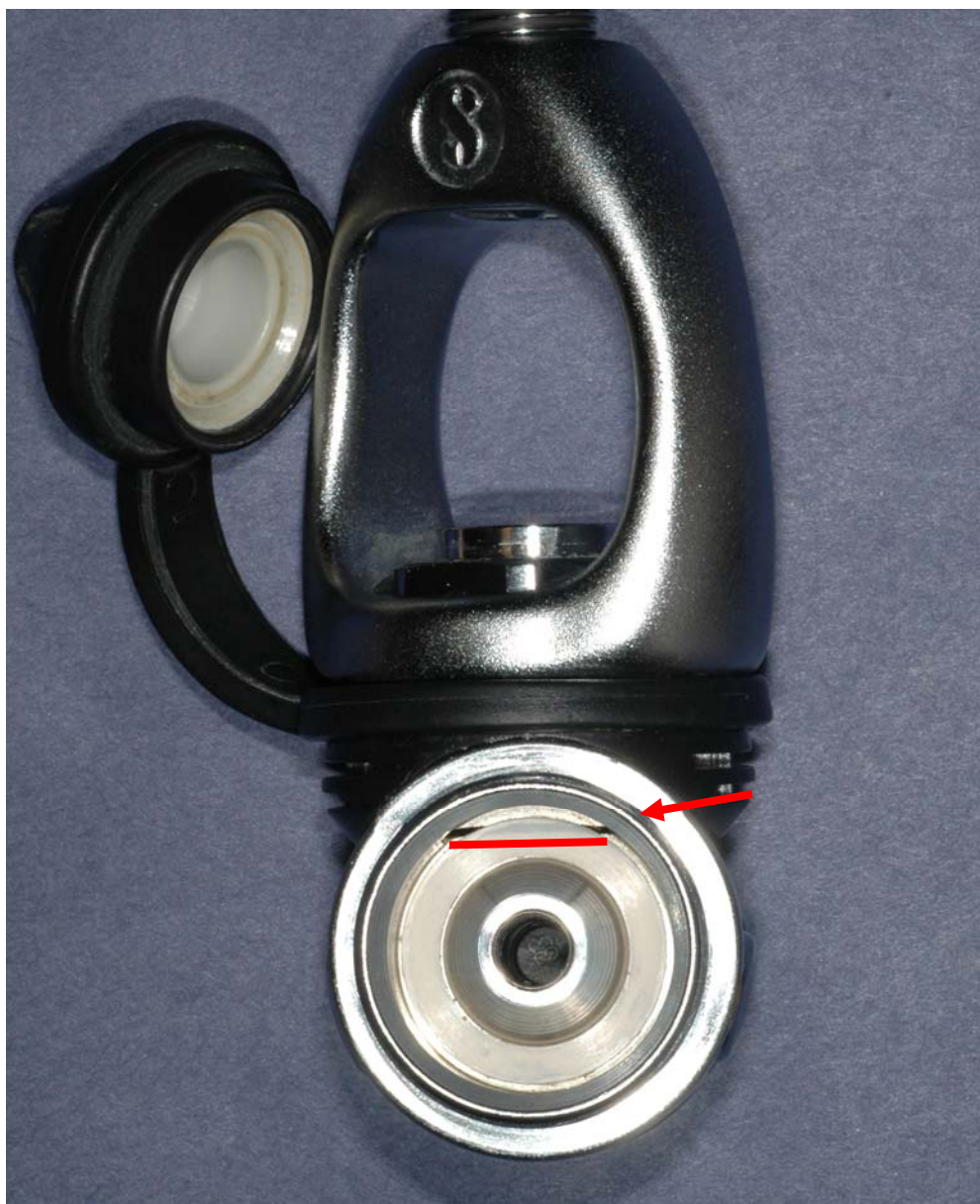
Figure 2. Detail of the view a service professional will have of the low-pressure side of the regulator body. If a pre-existing crack exists, it will be visible at the location of the red line in the photo. Service Technicians should add the inspection of this area (red line and arrow) during all MK20 service procedures and return any cracked components to SCUBAPRO for replacement.
