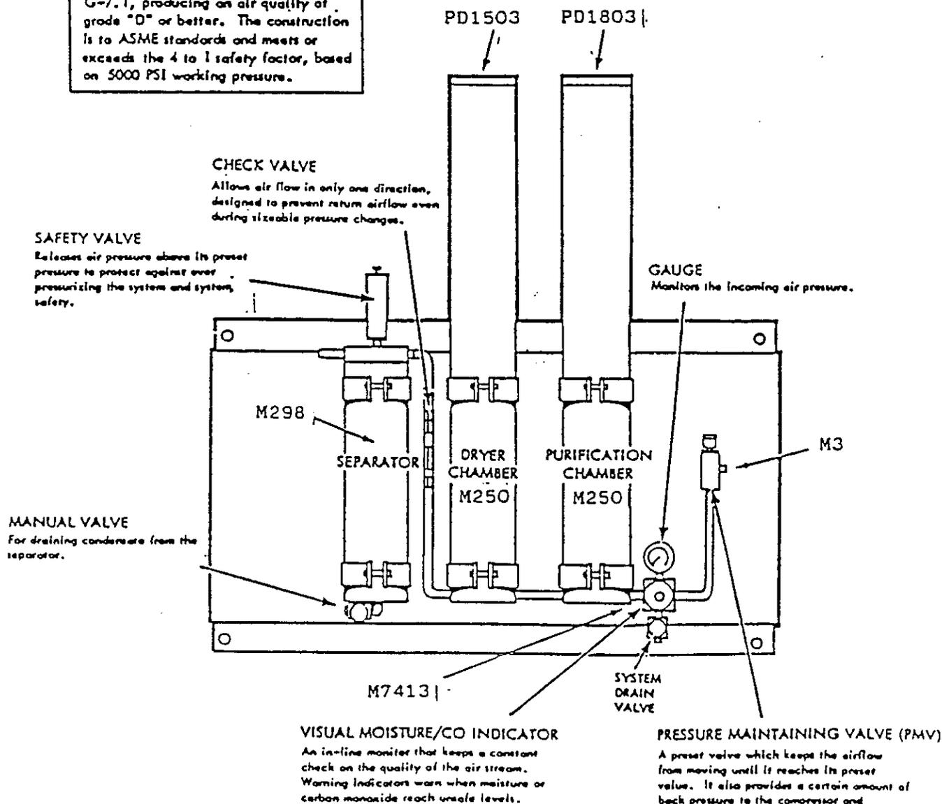
NOTE: The above drawing shows a wall mounted system. The location of the Moisture/CO indicator on vertical mounted units and details of it's operation are shown in succeeding pages.
