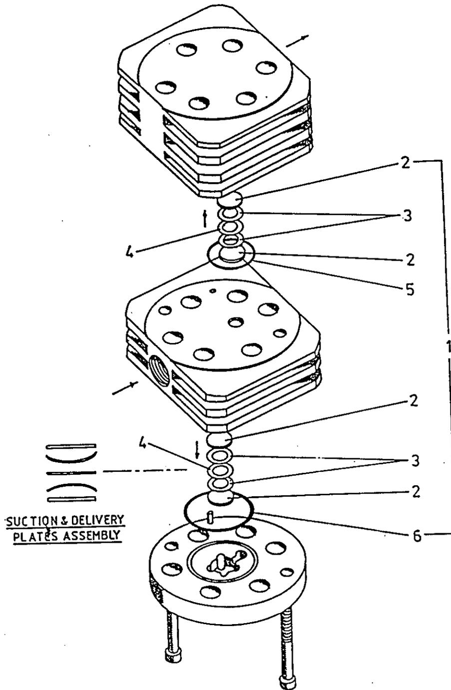
Figure 5-6 Valve, 3rd Stage, Inlet-Discharge
