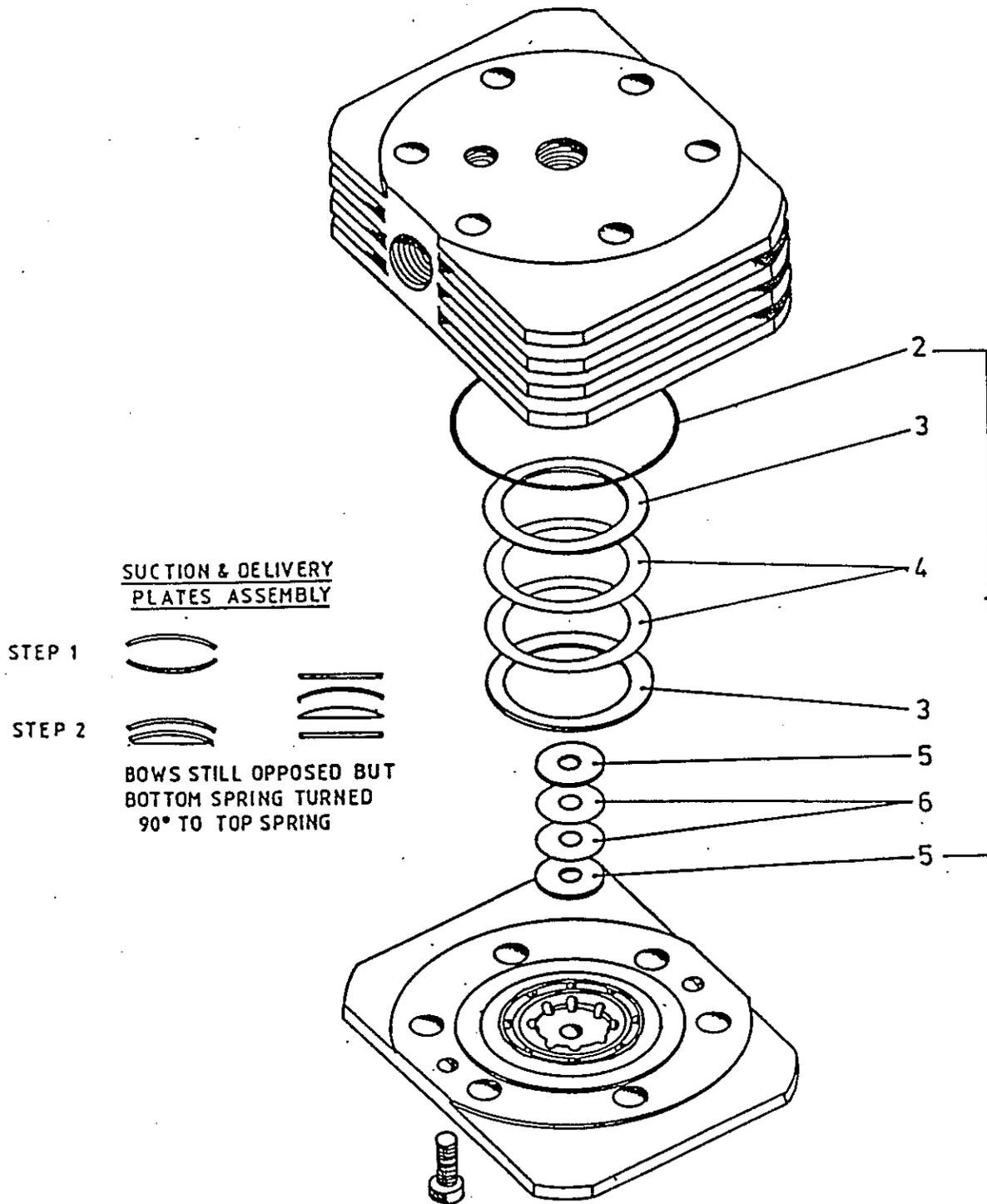
Figure 5-5 Valve, 2nd Stage, Inlet-Discharge
