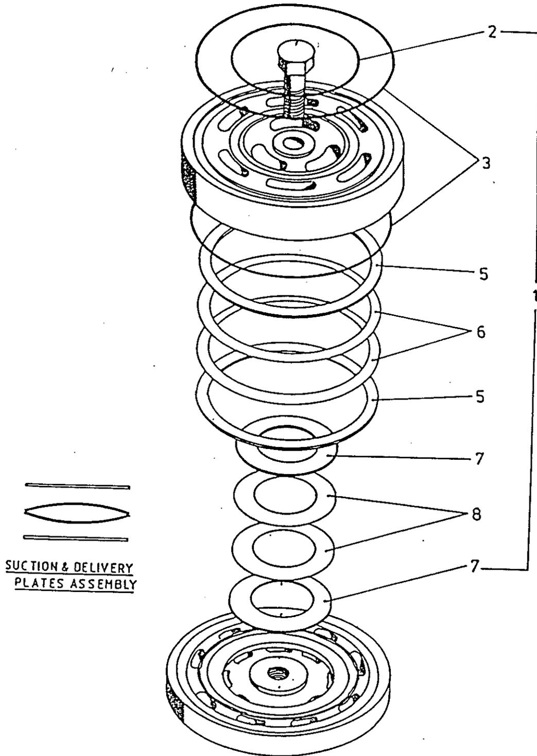
Figure 5-4 Valve, 1st Stage, Inlet-Dischrge K-7
