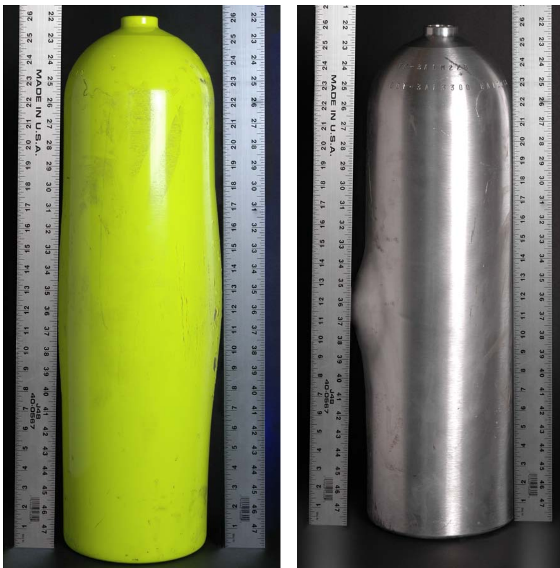
FIGURE 11: Bulged Cylinder
