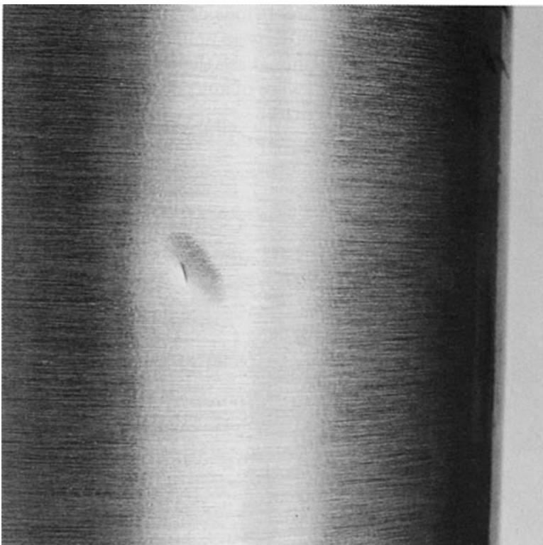
PHOTO 2. Gouged cylinder.
