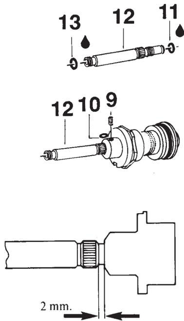
5. Install the o-rings (11,13) on the valve tube (12). Grease the threads and the o-rings.
