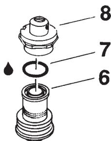
4. Place the valve housing in the handle. Tighten with a tool. See diagram.
