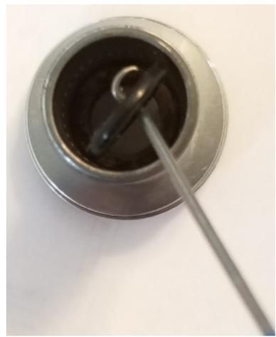
While the best example is retrieving the HP piston shaft o-ring from the bore of a classic Scubapro Mk10, the most common example where a double hook pick is invaluable is in retrieving the almost-invisible o-ring in a common bcd hose connection:
