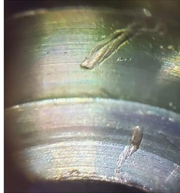
That's one reason that plastic and brass picks are so popular. They are softer than the chrome plating of your equipment, and are less likely to scratch it as a result. Still, spearing and sacrificing an o-ring with a sharp curved pick is still a standard technique for many technicians. But it doesn't take much to scratch the soft brass of a regulator body with any metal pick.
