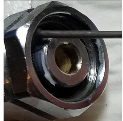
Now change the angle of the handle so the tip of the hook slides under the o-ring, and rotate the handle away until the sharp tip can just be seen on the other side of the o-ring.
