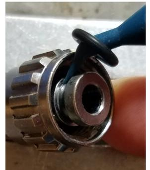
But at high pressures, it's a different matter. Scratching a similarly shaped groove inside an old Mk5 that you are trying to service will mean 3000 psi gas inevitably leaking into the ambient pressure chamber, giving you a bubbling first stage or worse. The o-ring has a harder duro (so as to handle the higher tank pressure) and is less able to mold itself to the scratched groove. Getting this o-ring out for replacement requires a double hook pick, and deft technique.
