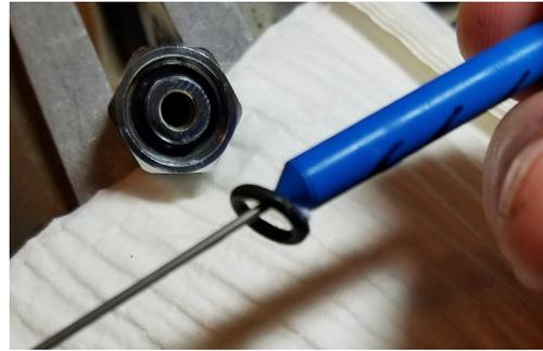
Working inside the bore of a piece of equipment is where a double hook pick is made to order. There's no room to slide the shaft of the tool under the oring, so the oring is carefully retrieved with the hook itself:
