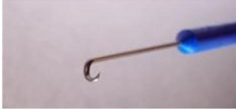
The reason the double hook pick exists is to reach inside a regulator or hose end to snag an o-ring that a straight or curved pick simply won't lift. Service manuals that specify a pick other than a double hook inevitably do one or both of the following: spear the o-ring, damaging it irretrievably, and/or scratch the groove of the equipment with the point. This old service manual photograph, and a picture of a balance chamber scratched while using its prescribed technique are perfect examples:
