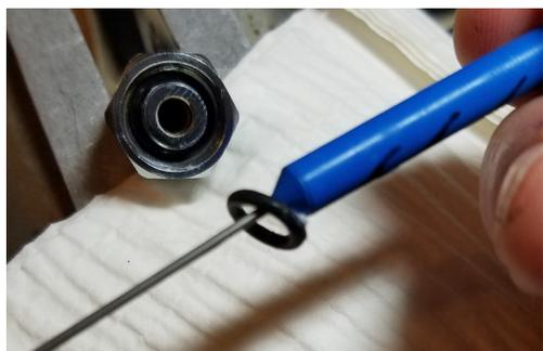
Sometimes, working inside the bore of a piece of equipment, there's no room to slide the shaft of the tool under the oring. In this case, the oring is carefully retrieved with the hook itself:
