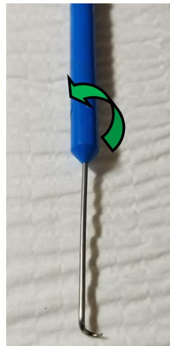
Properly using a double hook pick, then, requires making use of both the safe side and the right angle formed by the second hook. The pick is placed adjacent to the o-ring, by pushing it down into the land with the point protected. With the sharp tip lowermost (underneath the level of the o-ring), the handle is then moved to one side so the sharp tip passes under the o-ring but just above the land.
