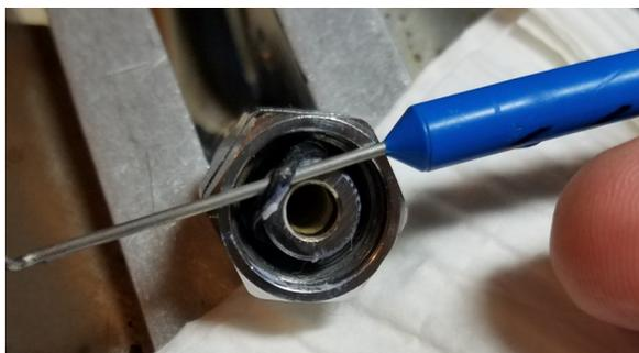
and then pop the oring out with the shaft of the tool.
