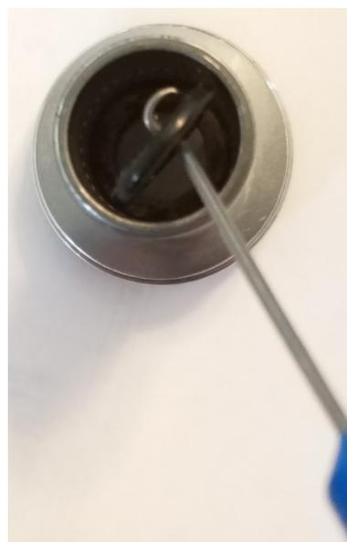
Remember that the point of the hook is harder than anything you're working on. Treat it like the dangerous weapon it is when inside your gear, and enjoy the ease with which otherwise difficult o-ring extractions can be made.
