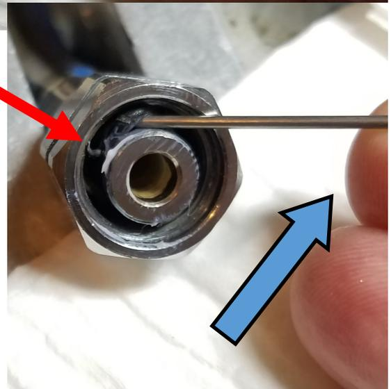
Rotate the handle even more away from you until the o-ring twists, and you can begin sliding the handle under the o-ring (to move the sharp tip away from both the oring and the equipment,
