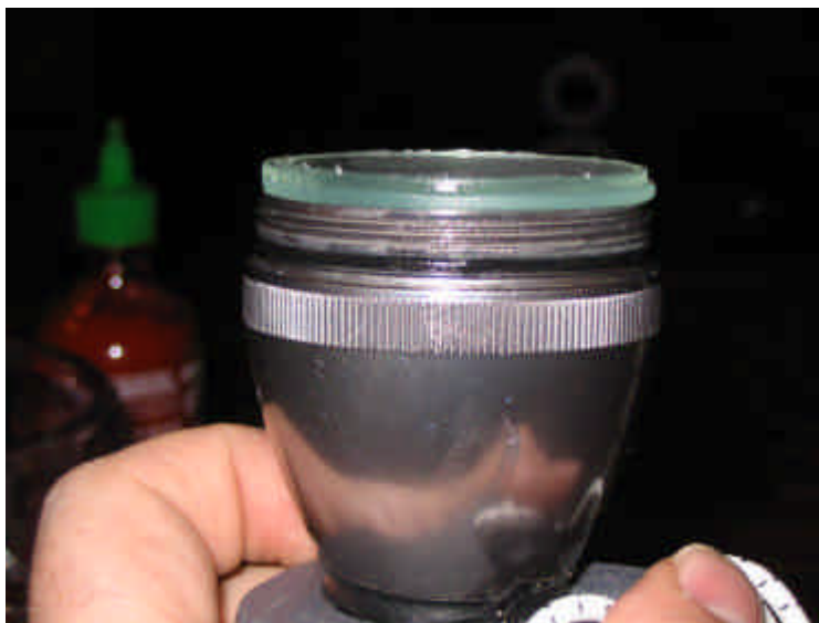
Figure 19: Double glass Maglite lenses seated atop MR16 bulb.
