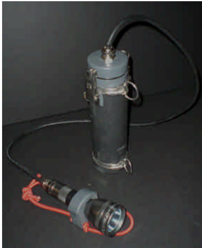
Figure 22: Heat shrink covered light. Note this light uses the magnetic reed switch, and does not require a switch on top of the lid.
