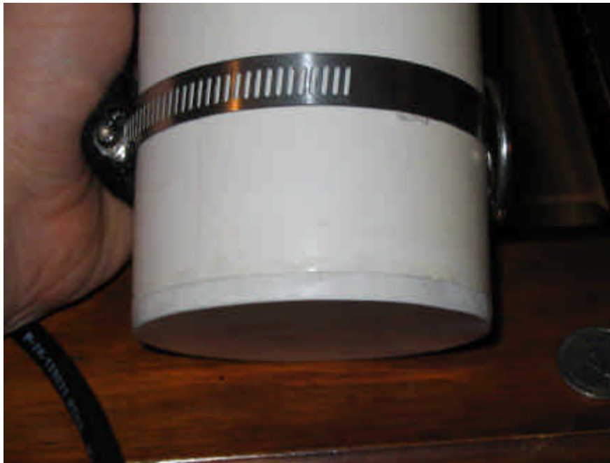
Figure 4: Cemented on end cap, sanded flush with bottom of the canister.
