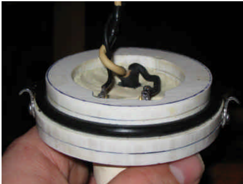
Figure 12: Bottom of lid bored out for switch.
