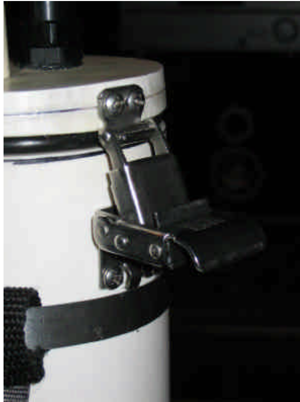
Figure 10: Proper latch orientation.
