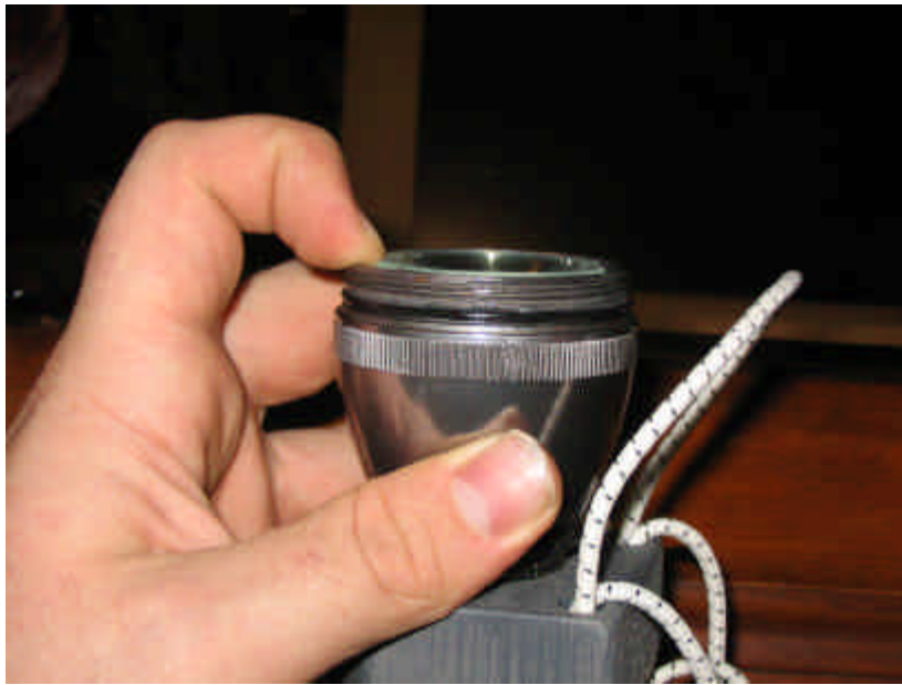
Figure 18: The MR16 bulb must be completely below the top of the threads.
