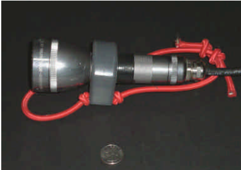
Figure 24: A magnet is mounted inside the PVC handle to activate the reed switch inside the lighthouse.
