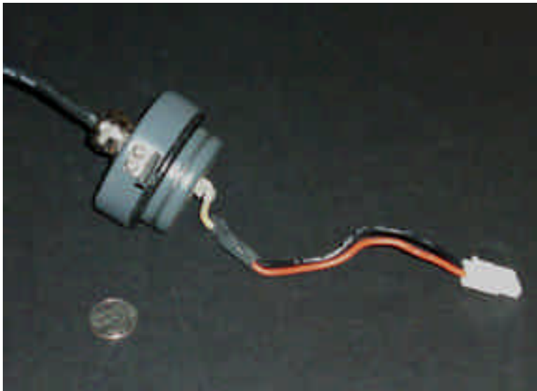
Figure 23: PVC round stock turned on a lathe to make a custom lid.
