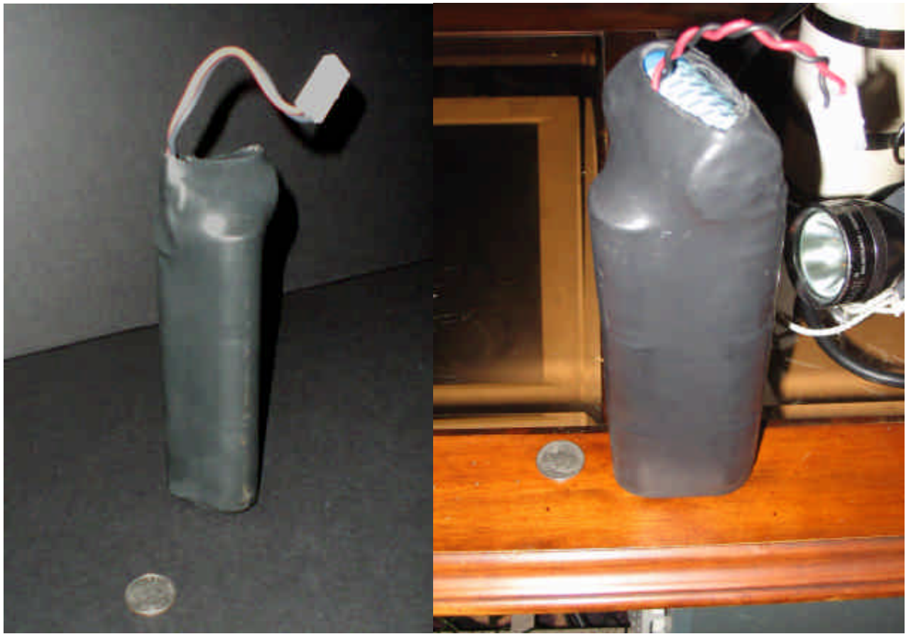
Figure 2: Assembled C-Size and D-size battery packs. Three columns of three with tenth cell horizontal.
