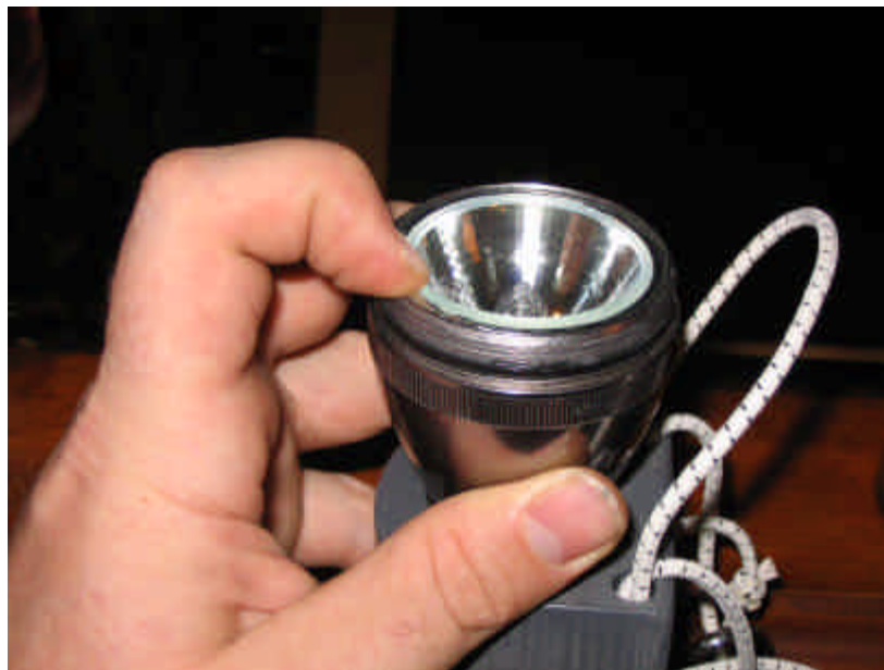
Figure 17: MR16 bulb inside of reflector assembly.
