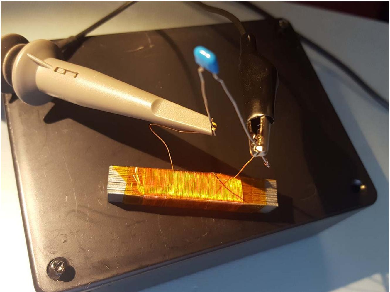
3. Transfer efficiency was much better when the xmit tank was driven by sine wave input: cleaner recv'd signal, stronger recv'd signal for lower xmit pwr. Also, matching tank resonant freq to signal frequency was less critical.
