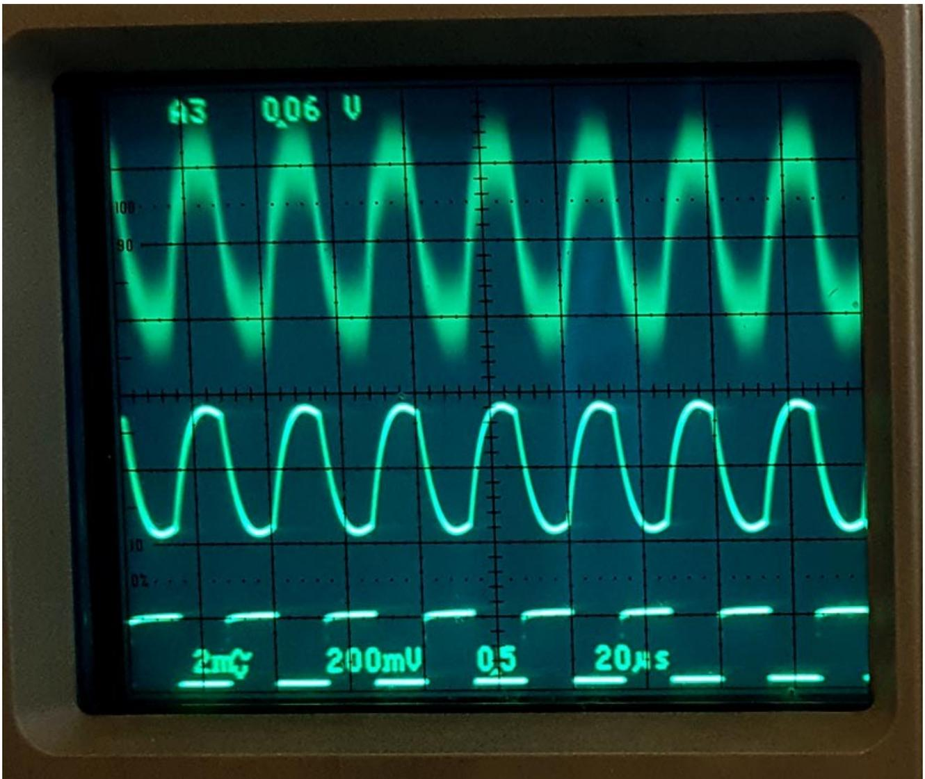
The gap between xmit and recv coils was just 3 cm for this test. Also, the signal gen output voltage was increased significantly in order to have about 3.5V P-P under load. Despite this higher xmit power and very short distance, the received signal was very weak and noisy (although still easily recognizable).
