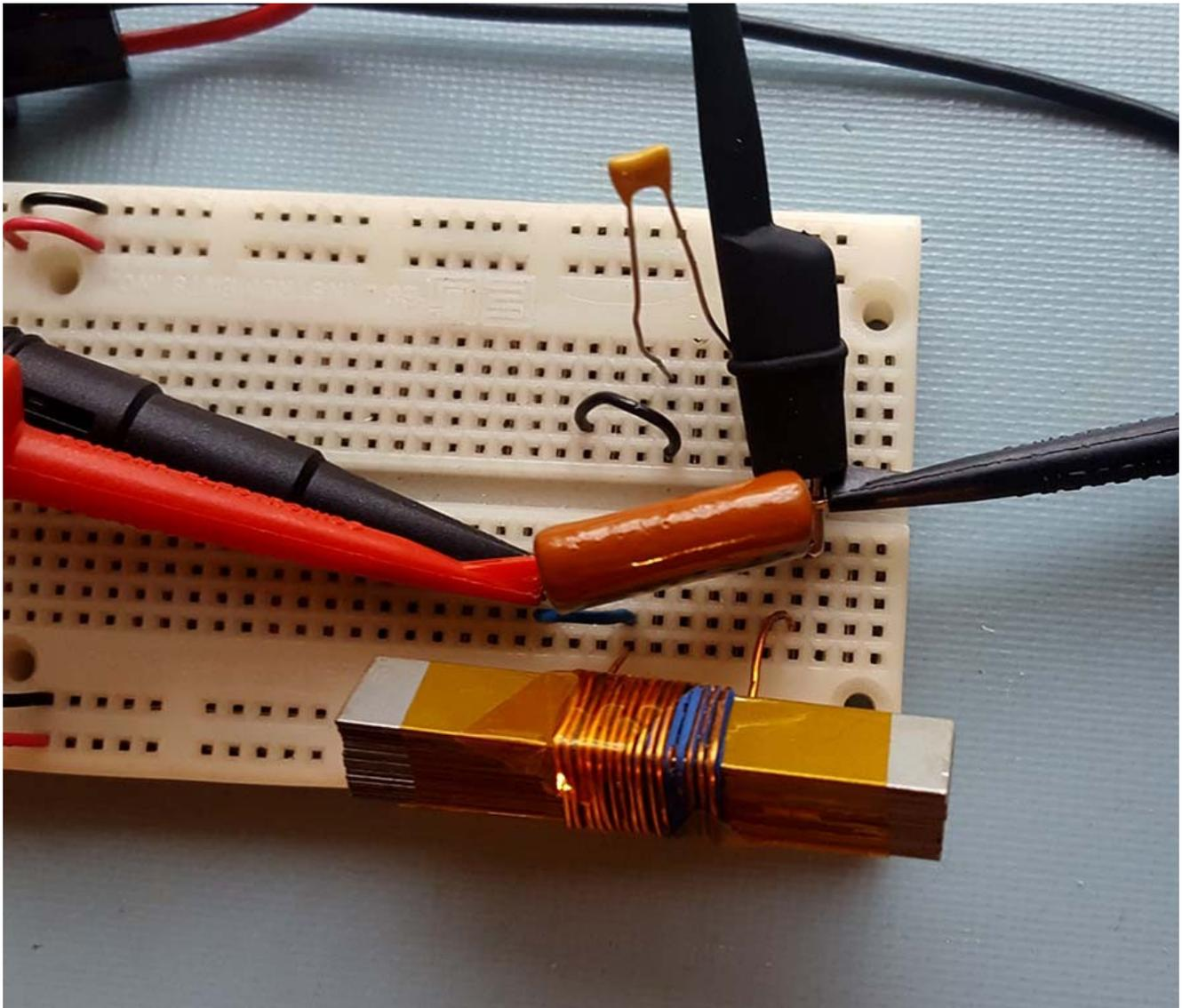
2. I saw much better performance with a low impedance xmit coil (fewer turns, larger diameter wire) but relatively higher impedance recv coil (many more turns, much smaller wire). DC resistance of my two coils is 0.145 ohm and 2.13 ohm, resp. Here's the receive coil. The recv cap is 0.047 microF.
