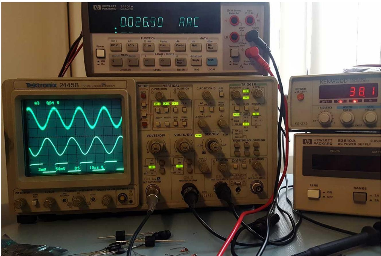
I set the no-load output voltage of the signal generator to 3.5V P-P, to simulate an average voltage in a transmitter using a single LiIon battery. As you can see the xmit tank has loaded that voltage down to 1V P-P; it is drawing 26.98 mA, and has filtered the applied square wave into a pretty respectable sine wave. The top trace shows that the induced voltage in the recv coil is about 4 mV P-P with just a little evenly distributed high-frequency noise.
