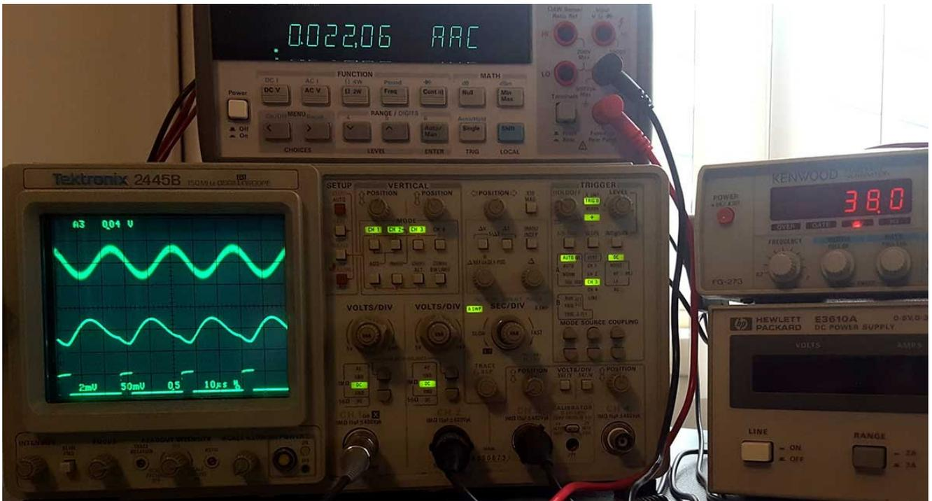
Although I had thought that it would be a good idea for the xmit coil to be a low impedance load (high current, stronger magnetic field) and for the rcv coil to be (relatively) high impedance, I was disappointed by my first tests. Here is an example trace.
