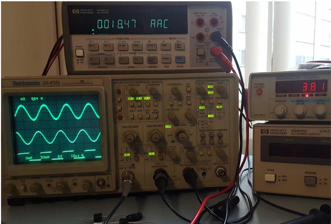
It's hard to see in the photos but the recvd signal is noticeably cleaner here. Finally, here are the traces when I reduced the square wave duty cycle to about 15% (this could be done to reduce power consumption at the cost of some signal integrity: more spurious transmission and lower S/N).
