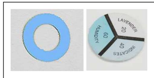
Colorimetry can be used to determine an end point value for your filter chemicals. If the one has a hour meter on the compressor, simply track the number of “running hours” since you last changed filters to the point where the humidity sensor fades from blue to pink. Repeat this procedure 3 - 4 times and take an average. This value is the “longevity function” of your chemical filters, or in simple terms, how long your filter cartridges will last as an average, measured in “running hours.”
