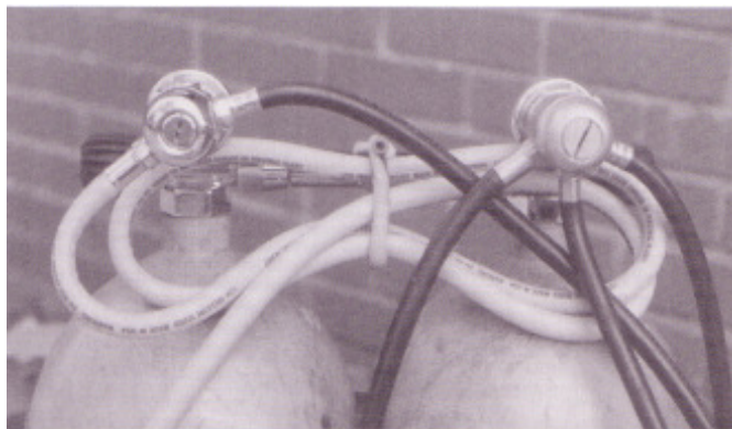
Figure 5-6 Coiled behind the neck storage.
