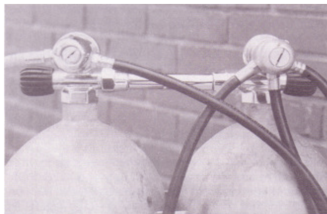
Figure 5-4C Streamlining using the same brand of regulators as Figure 5-4B, but with DVM with DIN fittings instead of yokes.
