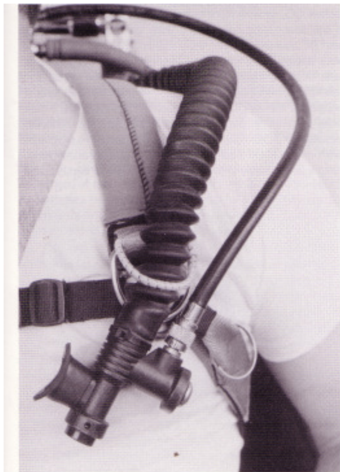
Figure 5-8A Inflator hose secured.
