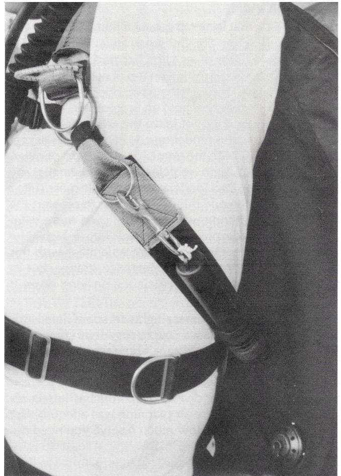
Figure 5-14A Hogarthian back-up light configuration: secured.
