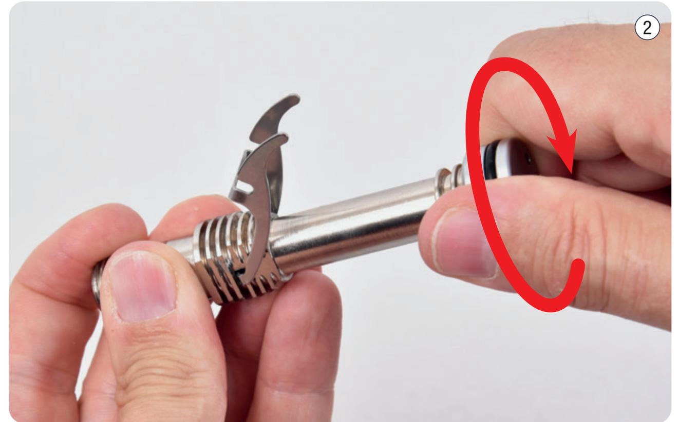
Insert the spacer into the valve body so that once it is screwed down, the valve body's flat wall will line up with the inside of the side cap. Screw the side cap for now; correct tightening is done in a later step.
