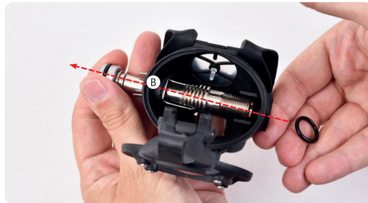
Press down the lever and simultaneously press (A) and pull out the complete mechanics of the 2nd stage, extracting it from the regulator case (B), as shown in the figure. Then remove the valve body OR from its seat.
