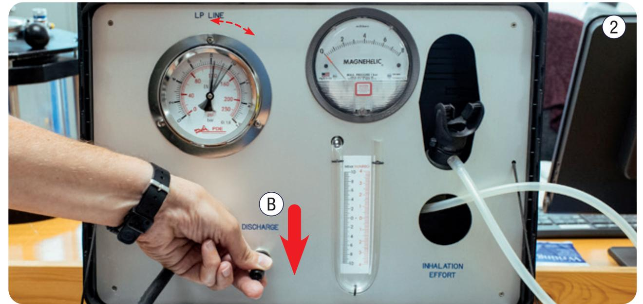
Once the regulator first stage is connected to the valve on the portable test bench, slowly open the air valve (B) (fig. 2), while simultaneously pressing on the test bench discharge lever (B) as shown in fig. 2 a few times to prevent the "water hammer" effect from occurring in the 1st stage HP valve and to stabilize the stage 1 set point value.
