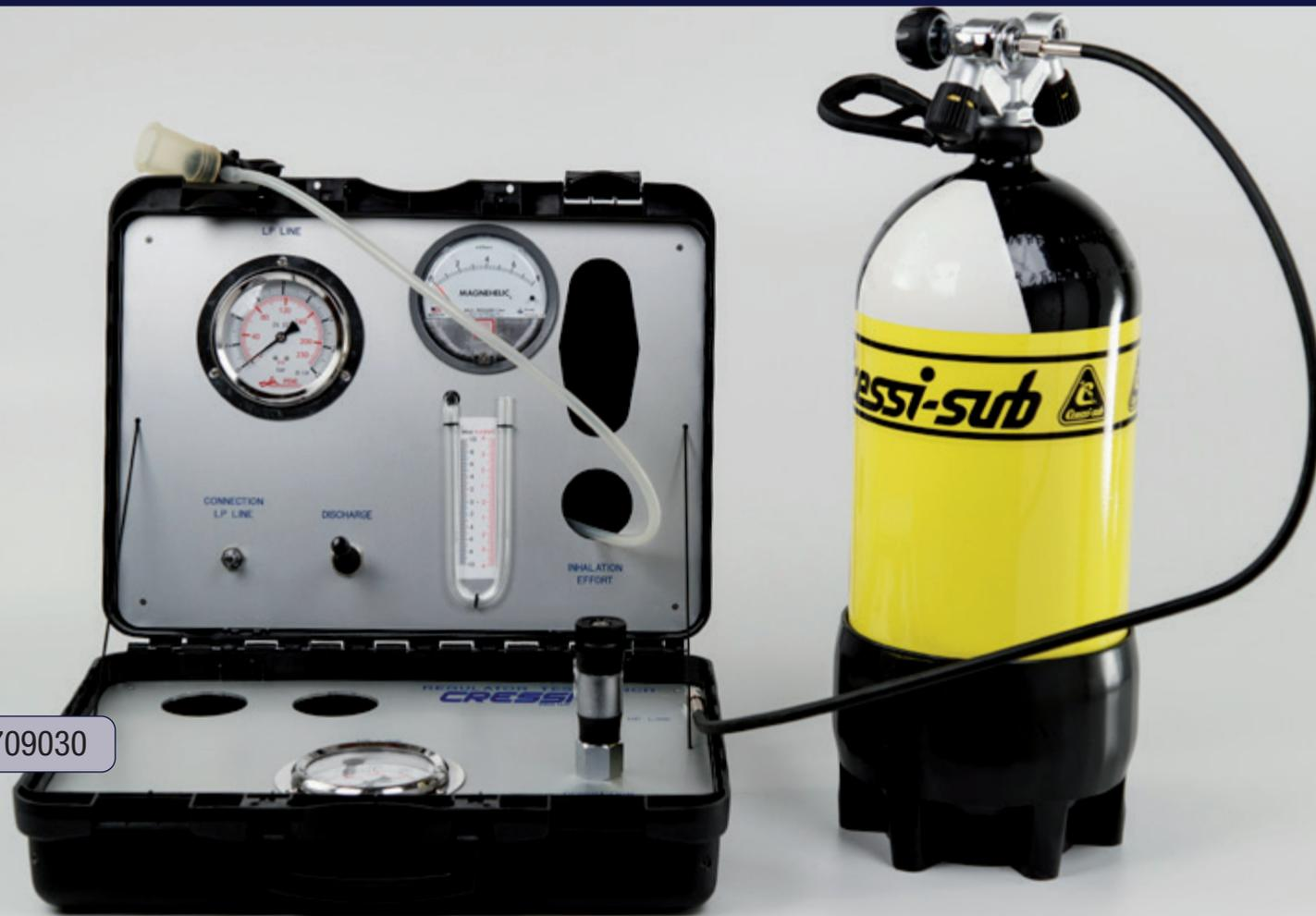
The most accurate regulator calibration is achieved using the portable Cressi test bench, code HZ 709030. Thanks to its pressure gauges with advanced reading class, it offers the possibility to calibrate both the first and second stages at the same time, providing a clear reading of the regulator calibration parameters, which otherwise remain entirely empirical.
