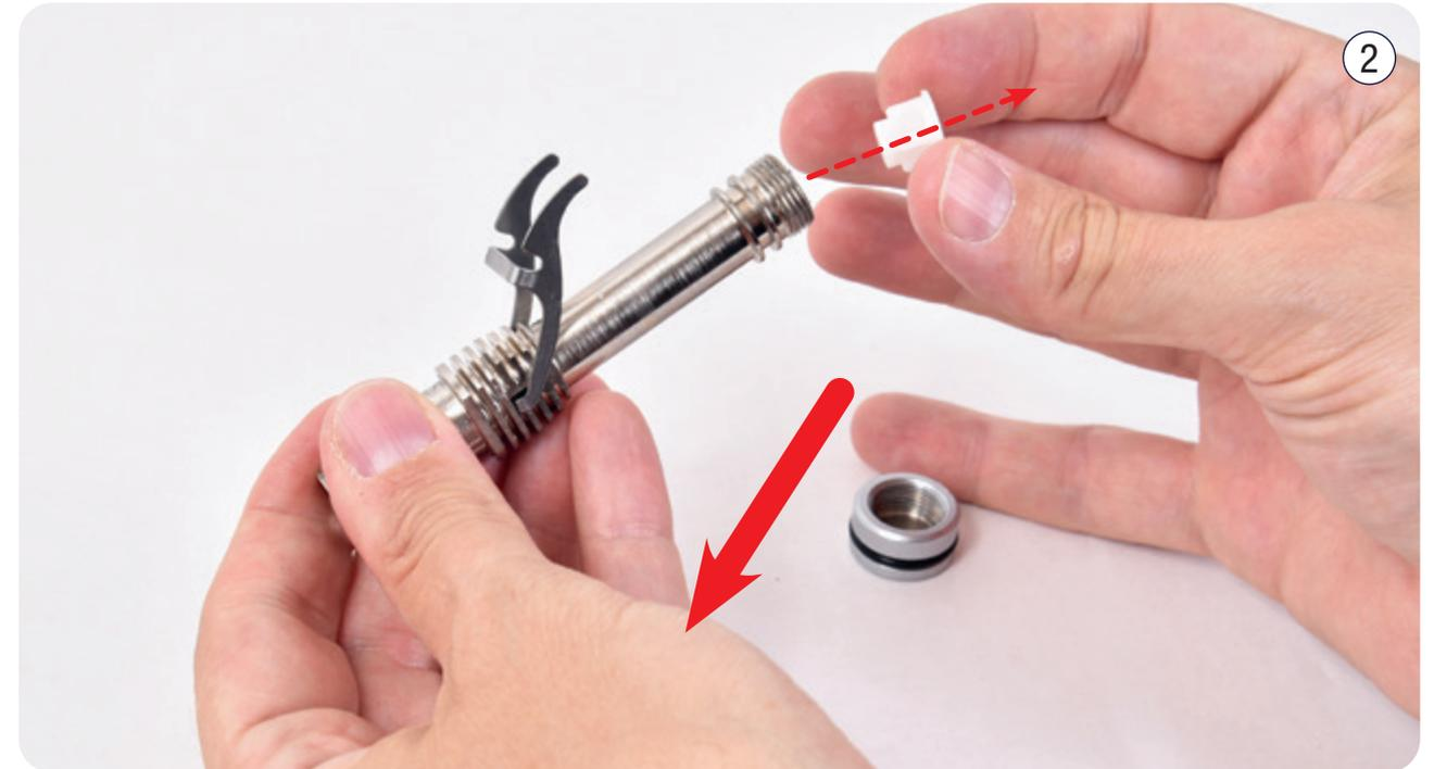
Remove the side cap, unscrewing it completely from the 2nd stage valve body (1). Remove the spacer from the 2nd stage valve body (2).
