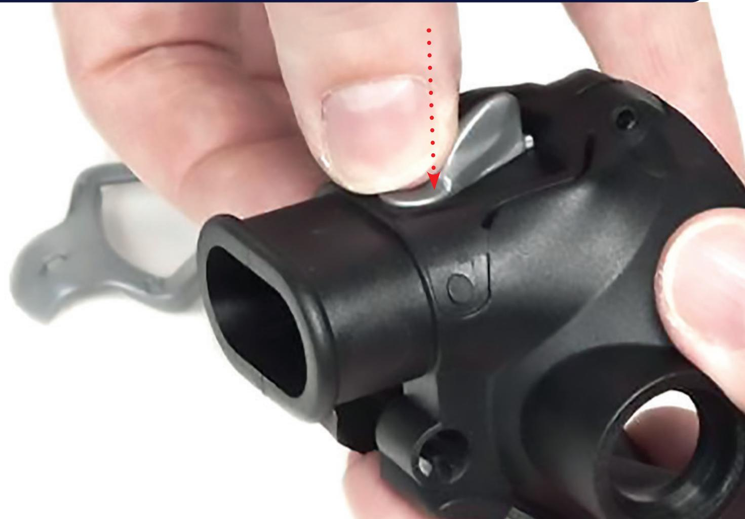
38 Insert the flow deviator into its seat as shown after you have replaced and greased the O-ring.
