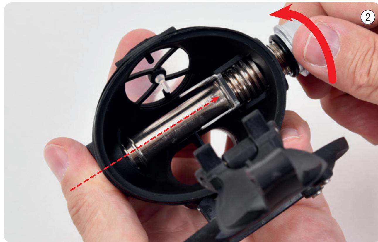
Replace and lubricate the valve body O-ring, and then position it in its seat as shown in the photo. Once tightened, a tab on the inside of the check nut titanium closing wall will ensure that the O-ring is seated correctly in position on the 2nd stage case.
