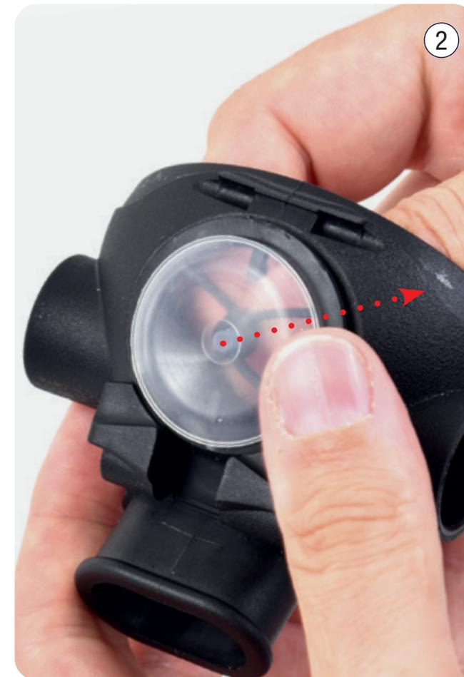
42 Insert the discharge valve (1), making sure to position the valve stem correctly in its seat, pulling it from inside the regulator (2).
