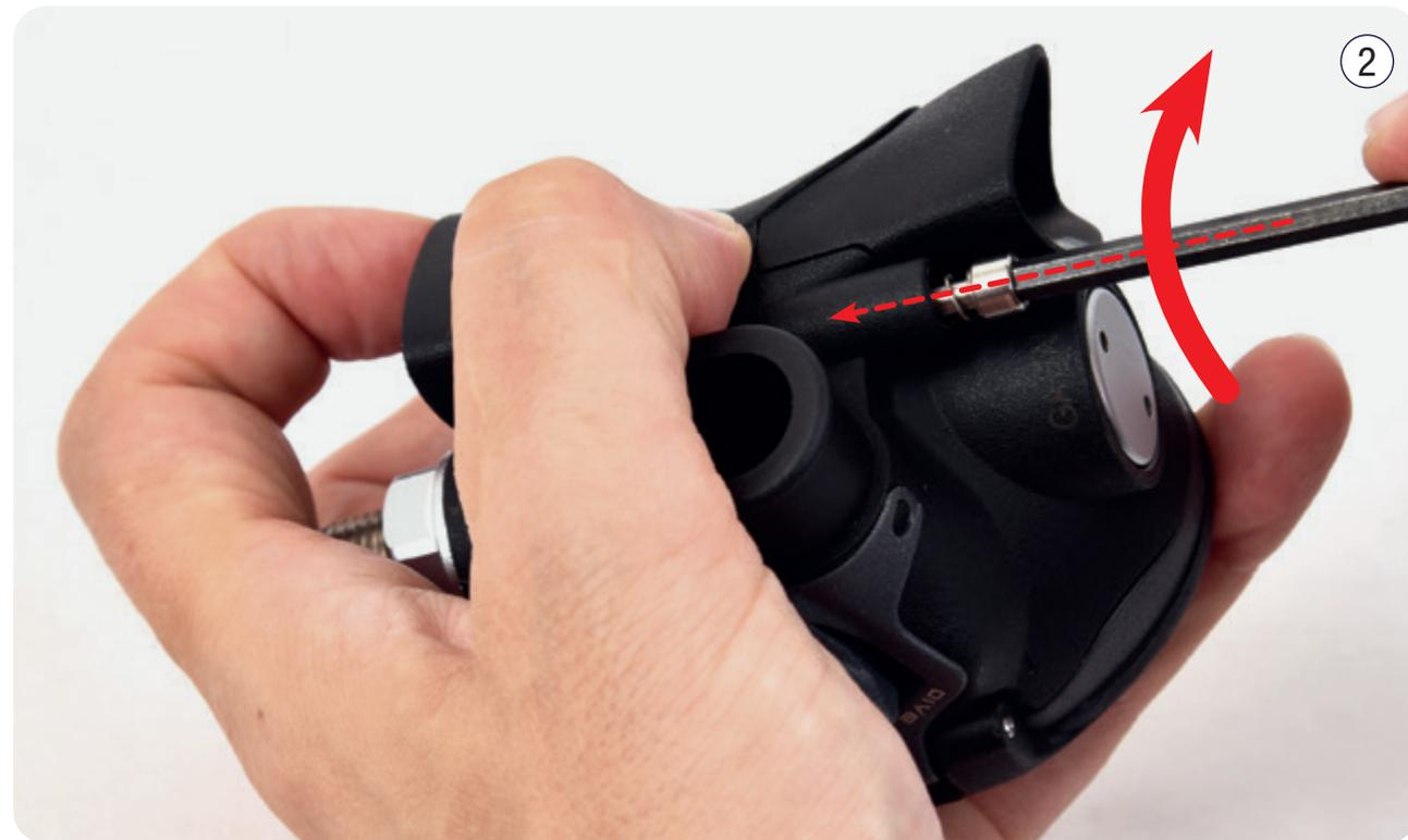
Position the "Cam-lock" in the direction shown in the photo. Then insert an Allen wrench in the corresponding socket, push gently, and simultaneously rotate 90° clockwise. The spring in the "Cam-lock" will push the key toward the regulator closed position, as shown in the photo.
