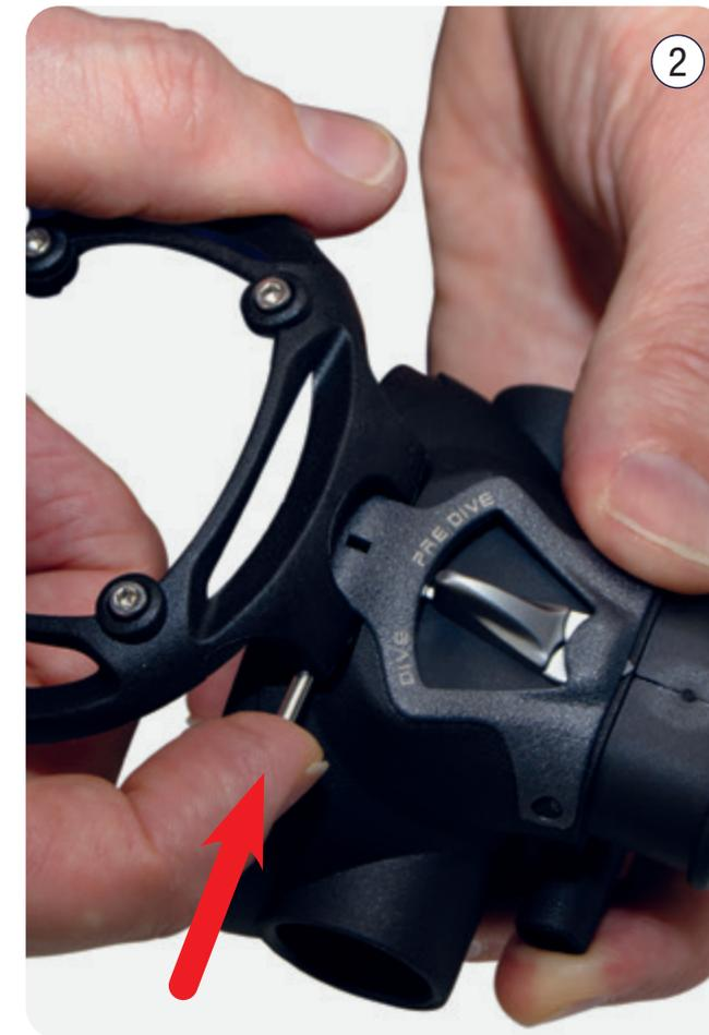
40 Insert the upper dome pin in the direction shown in the photo (1).
