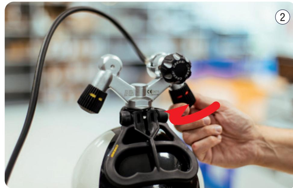
If this operation is done without the Cressi portable test bench, open the valve on the cylinder (1) (2) and simultaneously press the 2nd stage purge button (C) a few times to prevent the "water hammer" effect from occurring in the 1st stage HP valve and to stabilize the 1st stage IP value.
