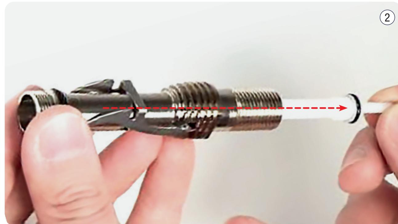
Extract the nozzle from the regulator valve body using the HZ 709011 tool (designed to prevent damage to the edge) as shown in the photo.
