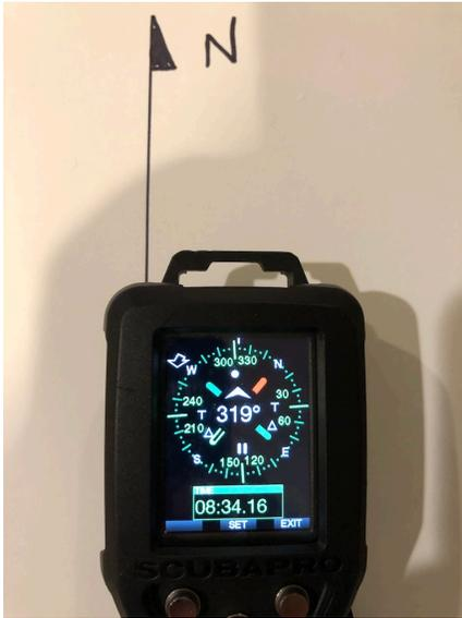
Turning 90 degrees. Even with the bad heading, turning 90 degrees does not give a 90 degree change of the incorrect heading. Correct heading shown by Scubapro FS2, Shearwater Petrel and Apple iPhone was 90 degrees. I would have expected the G2C to at least indicate 49 degrees which would be 90 degrees from the incorrect 319 heading. 90 degree turn is only showing a 53 degree change on the G2C.
