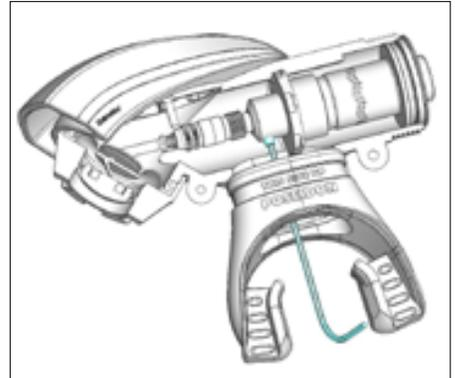
3) Alternatively: immerse the 2<sup>nd</sup> stage as shown in the illustration. A sizzling sound from the servo-valve opening shall occur within the two markings.
