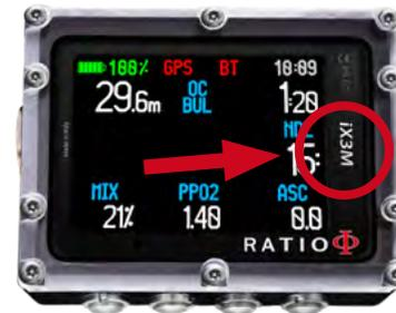
iX3M units that has "iX3M" only label on the top face can NOT be paired with the Ratio® CC Transmitter.
