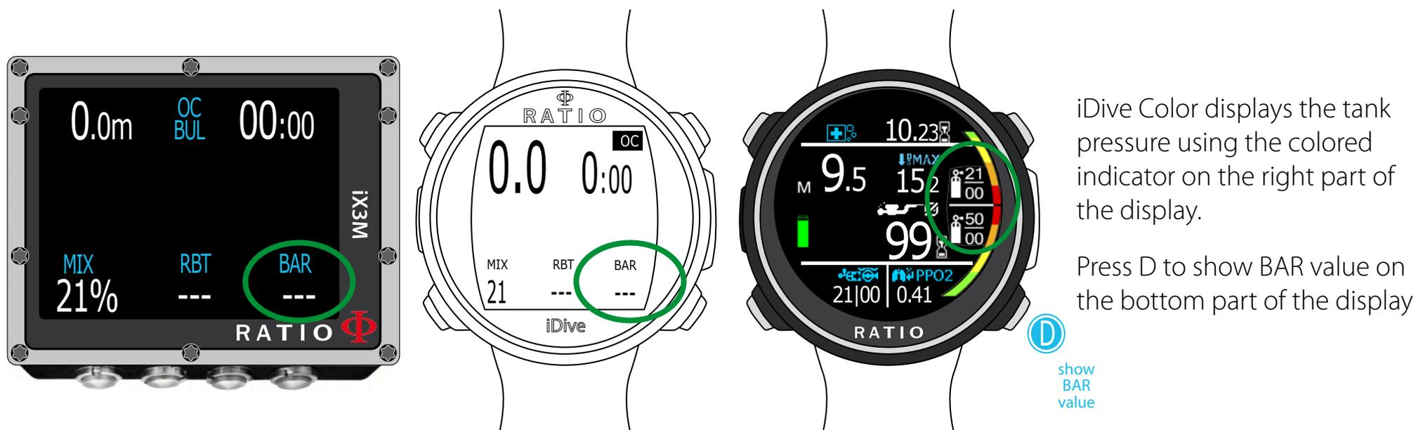
iDive Color displays the tank pressure using the colored indicator on the right part of the display.
