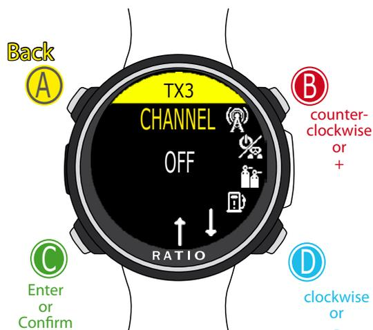
Place the iDive COLOR about 20-30cm from the CC Transmitter (Attention: If you place the CC Transmitter too close to the iDive COLOR the pairing procedure may not work properly).
