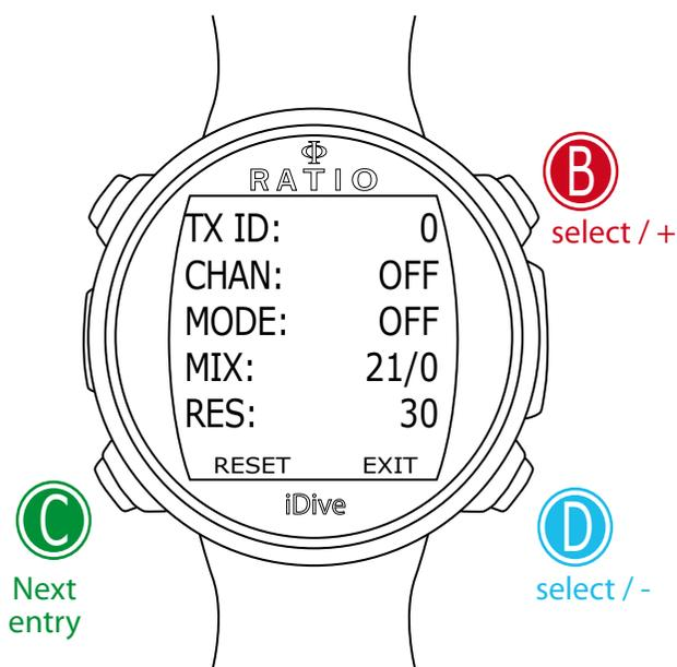
Place the iDive about 20-30cm from the CC Transmitter (Attention: If you place the CC Transmitter too close to the iDive the pairing procedure may not work properly).
