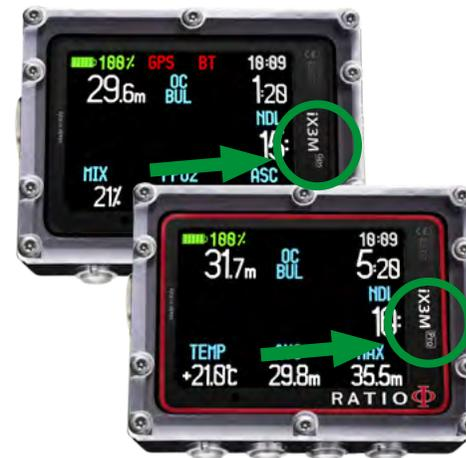
iX3M units that has "iX3M GPS" or "iX3M PRO" label on the top face can be paired with the Ratio® CC Transmitter.
