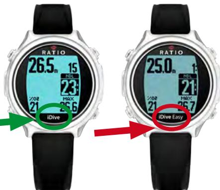
iDive Avantgarde edition units that has "iDive" on the top glass can be paired with the Ratio® CC Transmitter.
