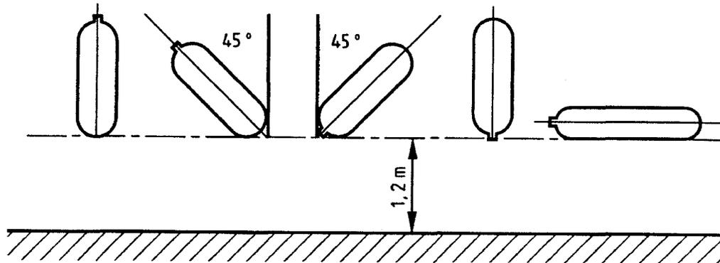
Figure 2 — Positions for the impact test
