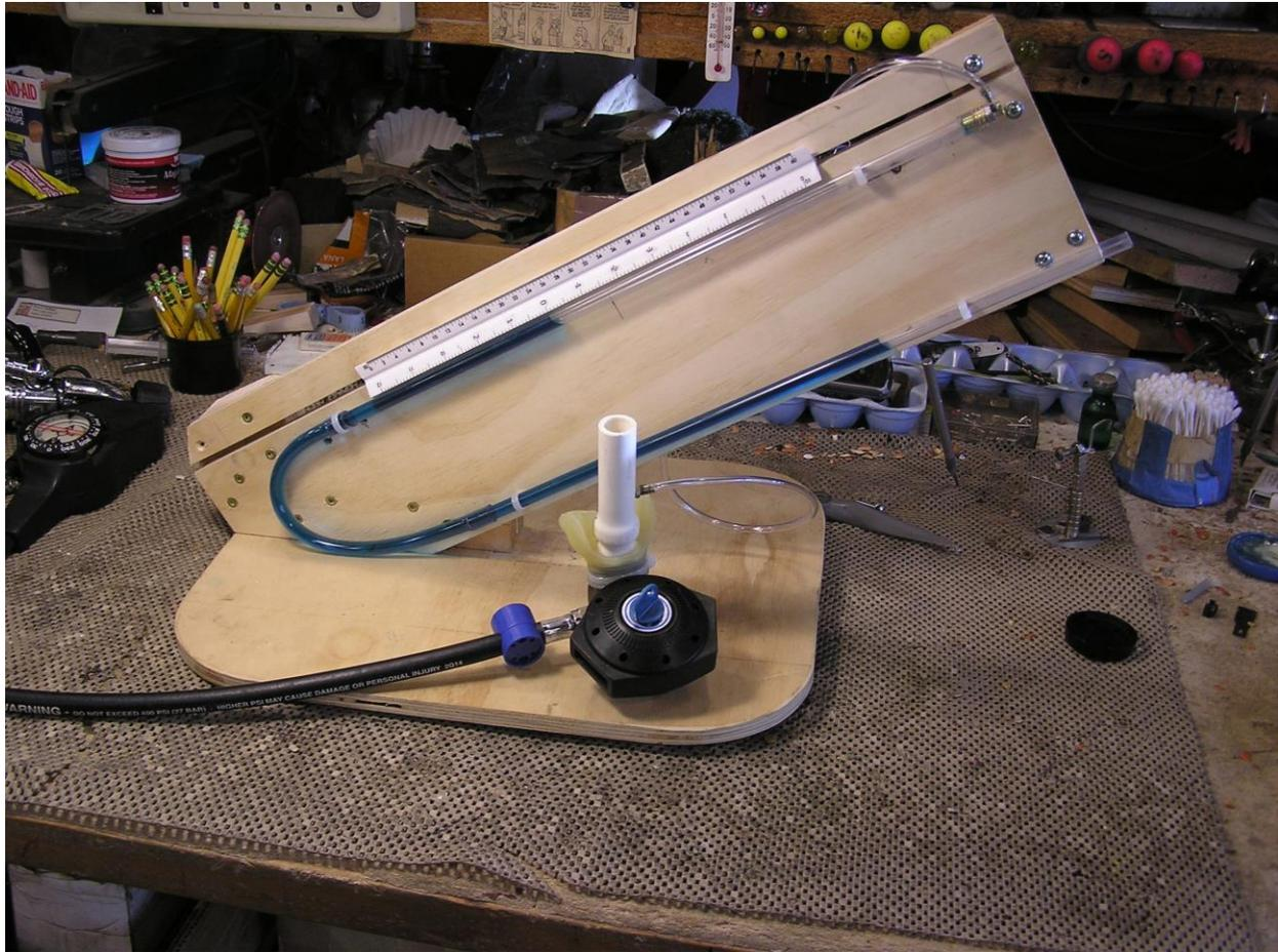
This is my DIY (Do It Yourself) slanted u-tube manometer. The water tubes are slanted at 30 degrees in order to double the scale reading for the difference in water surface heights (inches of water.) It works very well. I get accurate and repeatable readings. I can read to about +/- 0.05 inches of water.
