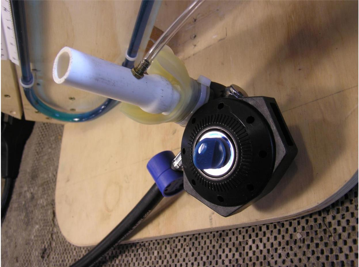
The regulator mouthpiece adapter is made from PVC tubing and connects the regulator to the upper end of the water u-tube with some vinyl tubing and a few fitting bits.
