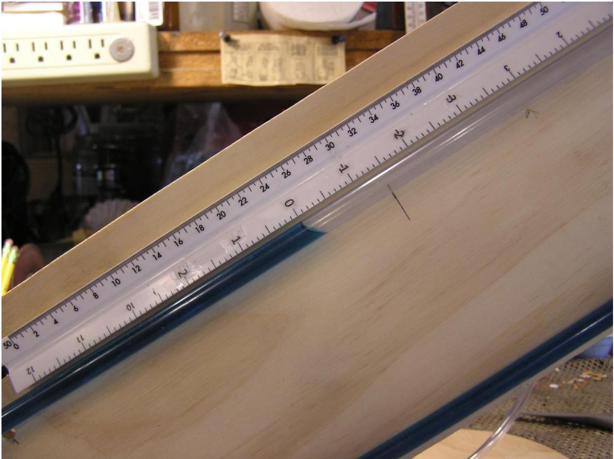
The scale I used has been remarked from plus 2 to minus 3 for ease of reading. The back edge of the scale is a snug fit in a slot in the wood frame so the scale can be slid up or down to align the scales zero-reading-point with the static water level in the tube. The tube has about a  $5/16$  inch (8 mm) inside diameter.
