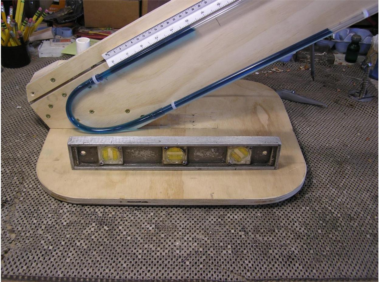
I use a level on the base when setting up to ensure accuracy.
