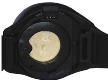
Battery compartment and pins for optional download cable.
