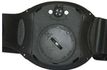
Battery compartment and port for optional download cable.
