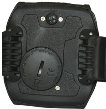
Battery compartment & port for download cable.
