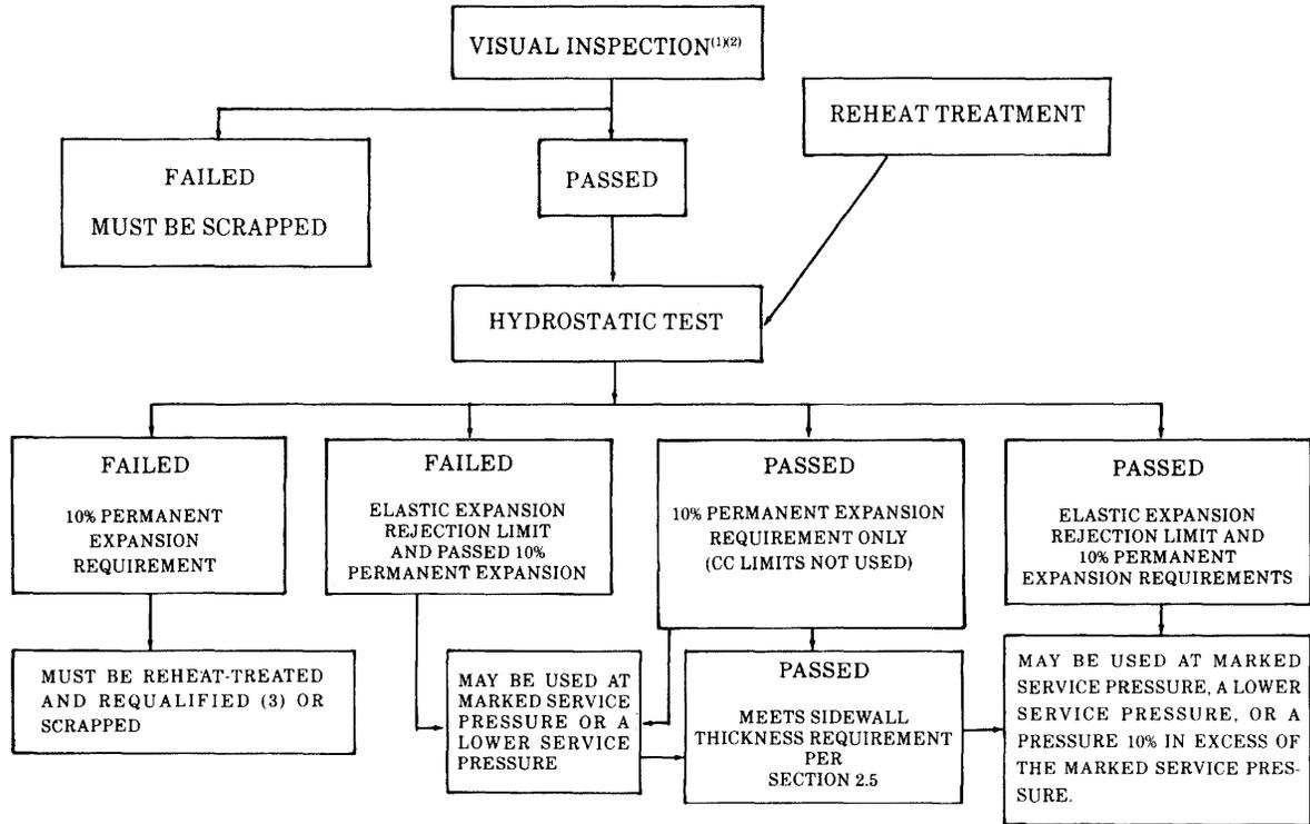
(1) Visual inspection must be conducted in accordance with Compressed Gas Association C-6 [2].
