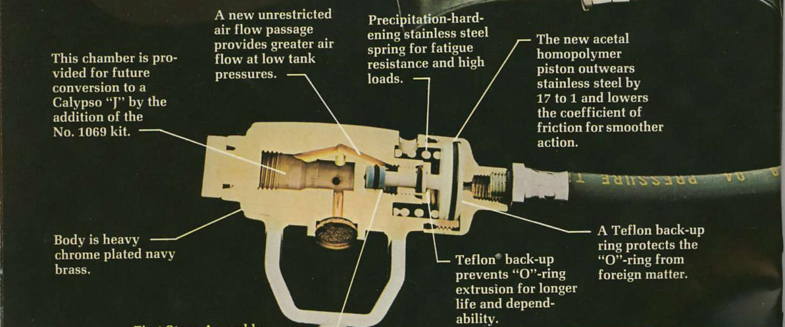
The new acetal homopolymer piston outwears stainless steel by 17 to 1 and lowers the coefficient of friction for smoother action.
