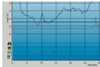
Smart TRAK displays the ppO<sub>2</sub> limit as a black bar on the graph at the depth at which the ppO<sub>2</sub> limit is reached. In this instance for a 33% mix at 1.4 bar it is 105 ft (32 m).
