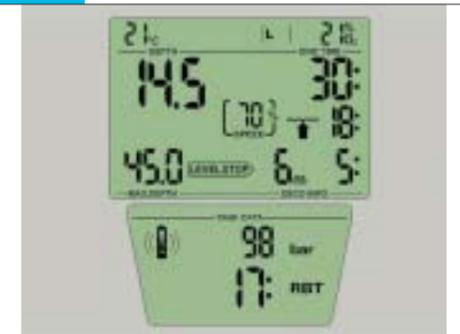
Smart TRAK replays actual screen data for the Smart COM and the Smart PRO in 4 seconds intervals.
