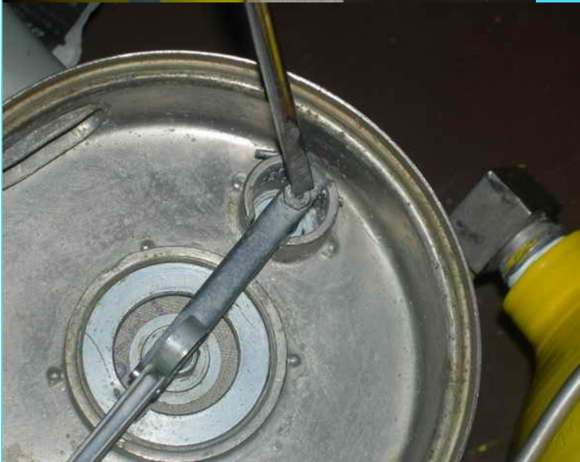
After all adjustments, we put the pulmonary automatism diaphragm, cover and tighten everything with clamps.
