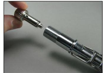
22 Using the seat extraction tool, carefully push the crown (16) out of the valve body (19).
