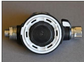
**CAUTION:** Make sure the diaphragm washer is completely flush with the edge of the case. Confirm the diaphragm is not pinched.
