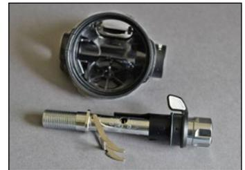
**11** From the left side of the case (8), remove the spacer (13) and oring (14).
