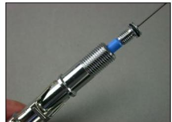
23 Remove the crown oring (15). Critically inspect the crown (16), paying special attention to the sealing area as well as the oring groove.
