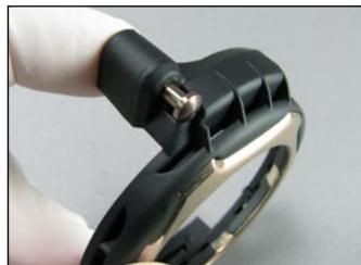
**24** Press the metal ring (2) into place on the front cover (1).
