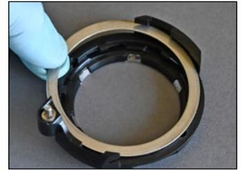
**25** Position the front cover (1) onto the case (8). Lift up the pin locker and rotate the front cover clockwise until the pin lines up with the hole in the case. Release the pin when lined up, it should move into the hole in the case.
