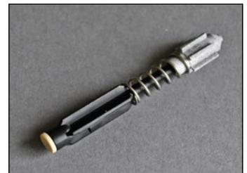
**4** If you removed the lever (20), replace it on the valve body (19) so that the lever is on the side with the small dot as shown in this picture.
