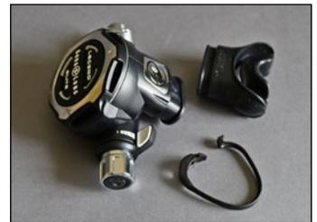
**5** Lift the pin locker all the way up, rotate the front cover (1) counter-clockwise until the pin is clear of the case (8). Remove the front cover.
