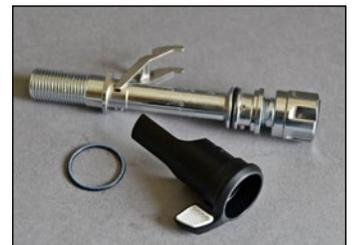
**13** Turn the adjustment knob (29) ½ turn clockwise allowing the pin (21) to fall out. If the pin does not fall out, use an oring removal tool to carefully push it out. Turn the adjustment knob counter-clockwise and remove it from the valve body (19).
