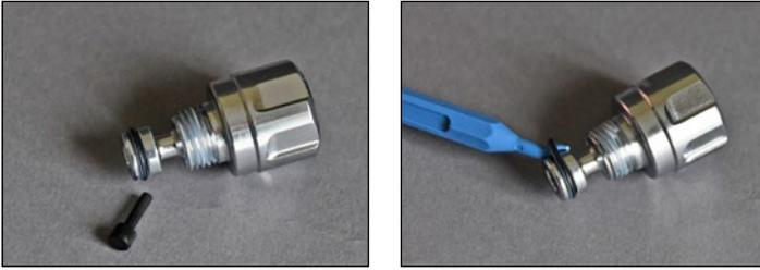
15 Using a hooked oring tool, insert the point into the small hole in the center of the plug (32). Carefully pull the plug out of the adjustment knob (29).
