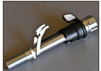
**11** While depressing the lever (20), insert the valve body (19) through the right side of the case (8). Do not allow the lever to spring up forcefully as it passes into the case.
