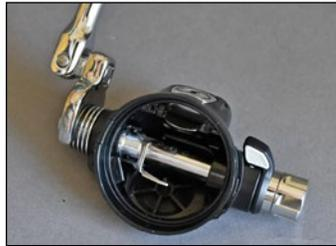
**15** Fit the o-ring (15) onto the crown (16). Press the crown, threaded end first, into the valve body (19). Use the crown adjustment tool (RG911137) to push the crown into the valve spindle as far as it will go.
