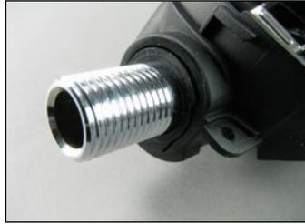
**14** Thread the heat exchanger (12) onto the valve body (19) until finger tight. Using a torque wrench with a 19mm (3/4") crow-foot, tighten the heat exchanger to a torque of 45 in-lbs (5 Nm).
