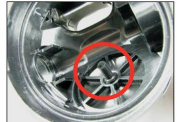
**2** Carefully push a new MP seat (22) into the shuttle valve (23). Make sure the seat is flush against the valve. Install oring (24) onto the shuttle valve, put some extra Christo-Lube on the end of the shaft.
