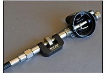
**CAUTION:** Prior to adjusting and testing this second stage regulator, the accompanying Leg3nd first stage must be correctly serviced, and adjusted to the proper medium pressure 116-130 psi (8-9 bar) and fully tested. Refer to the appropriate first stage service course for any needed adjustments to the first stage before attempting to perform the adjustment and testing of the second stage.
