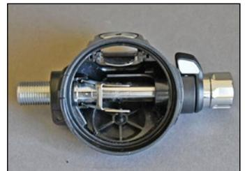
**CAUTION:** Do not allow the lever to spring up forcefully as it passes through the case. This could cause the lever to disengage from the shuttle valve, requiring disassembly of the valve body assembly.
