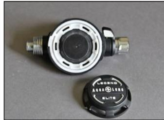
**8** Using your finger, lift up on the tab to remove the diaphragm washer (4). Carefully remove the diaphragm (5).
