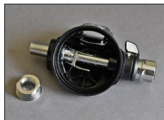
**10** While keeping the lever (20) depressed, pull on the adjustment knob (29) and remove the valve body assembly (15-32) from the case (8).
