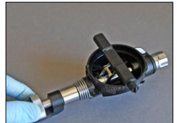
**a If an airflow exists:** The lever is set to high. Press inward on the adjustment wheel of the inline tool. Slowly rotate the adjustment wheel until the inline tool engages the crown (16). Turn the crown clockwise until the lever drops (20). Adjust until the lever is touching the bottom of the tool.
