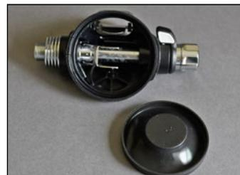
**9** Turn the adjustment knob (29) counter-clockwise until it stops. Using an 19mm (¾") wrench, turn the heat exchanger (12) counter-clockwise to loosen it. Once loose, unthread by hand and remove it from the valve body (19).
