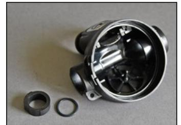
**12** While holding the lever (20) down, carefully slide the venturi (18) off of the valve body (19). Remove the oring (17) from the venturi.
