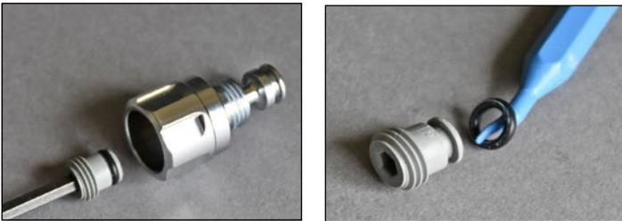
17 Remove the oring (14) from the valve body (19).
