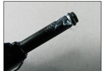
**3** Fit the spring (25) onto the leading edge of the counter-balance chamber (26). Carefully guide the stem of the shuttle valve (23) through the spring and into the counter-balance chamber.
