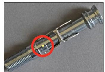
**5** Install o-ring (14) onto the valve body (19). Install oring (28) onto the adjustment knob (29)
