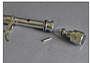
14 Remove the pin (27) from the adjustment knob (29) by tapping or shaking the knob. Remove the oring (28) from the knob.
