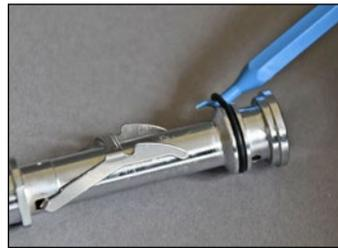
18 Using a 4mm hex key, insert it into the threaded end of the valve body (19) and carefully push out the shuttle valve assembly (22-26).
