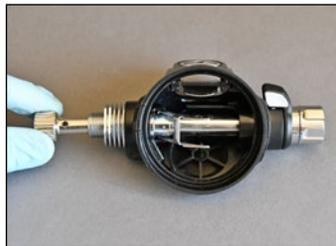
**16** Confirm the adjusting knob (29) is all the way out. Hold the case (8) so that the rim is at eye level. Using the crown adjustment tool (RG911137), turn the crown (16) in (clockwise) until the lever (20) drops about 4mm below the case rim. Then, turn the crown counter-clockwise until the lever is just visible above the case rim. This is a preliminary setting only.
