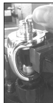
Yoke screw enough screwed
