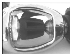
Yoke screw not screwed enough
