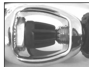
Yoke screw enough screwed
