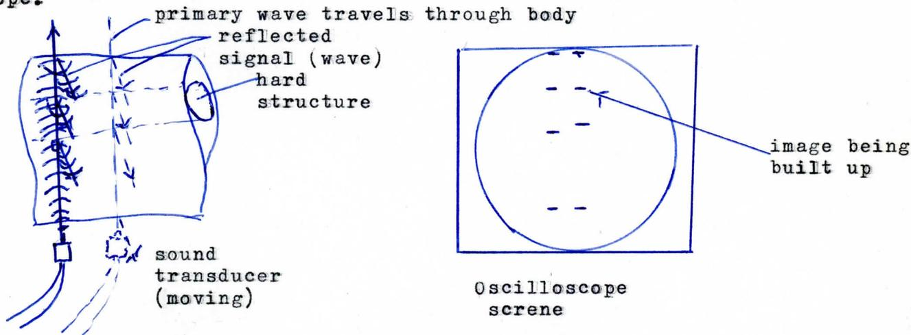
The sound transducer uses 5000 cycles/second frequency and this is shown on the oscilloscope at 20 scans/second.
