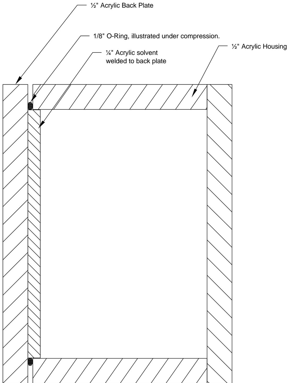
Typical DIY underwater Acrylic housing back plate seal design fabricated with a table saw. Cut the  $\frac{1}{4}$ " plexi for a close slip fit into the housing and slightly round sharp corners to prevent O-ring damage.
