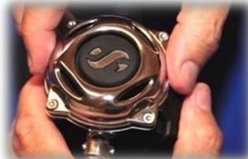
36. Align the cover (with screws and o-rings already installed).
