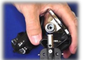
27. Fully engage function #7 into the back slots of the adjustable orifice. Unscrew counterclockwise, until threads have disengaged, (approx. 4 rotations).
