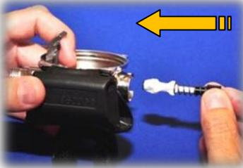
13. Pre assemble the poppet, spring and balance chamber. Orient the pair of “poppet shoulders” (down) in relation to the lever (up) and insert into the case inlet tube.
