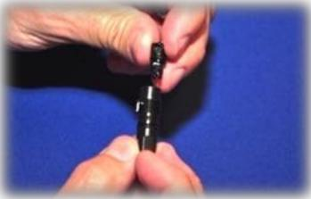
17. Push "micro adjust" into the "adjustment shaft" and hold with finger-pressure.
