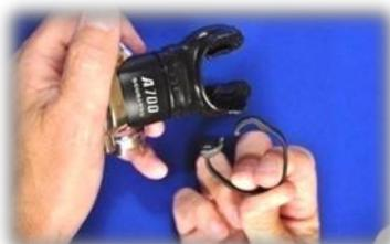
2. Spread and fasten the specialized hook and lock clasp. (Cam action). Note: Position the clasp opposite the "dive switch", avoiding interference.
