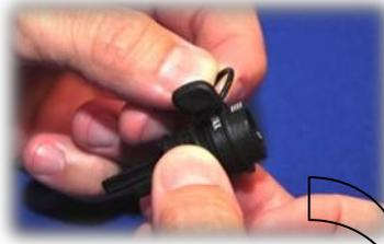
22. Prep the "dive switch" by installing both o-rings supplied in the maintenance kit.
