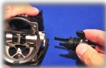
25. Place the "dive switch" assembly into the case. Orient the long-tab (towards the mouthpiece) and engage into the "flow deflector-guides".
