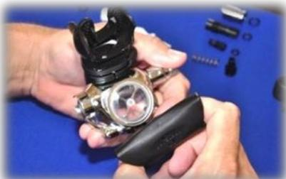
Note the position of the index figure and thumb inside the ends of the exhaust T.
