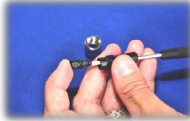
17. The *technician* micro-adjust is concealed within the knob stem and is driven out clockwise, using a small flat blade screwdriver.
