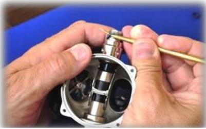
31. Remove inlet tube o-ring.
