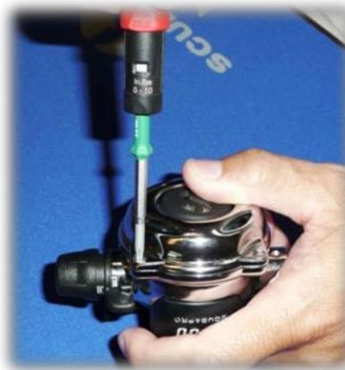
38. Using Torque driver, tighten the screw to the recommended 6.2 inch pounds / 0.7 Newton meters. See tool list on page 2 of this manual.
