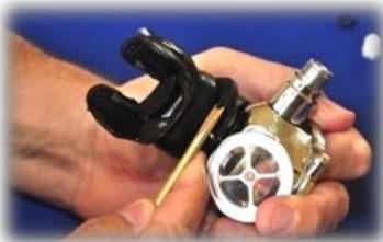
34. Remove the mouth piece by "releasing" the specialized clamp locking device. **See next image for more detail...**
