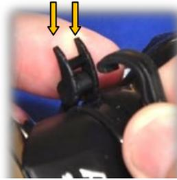
35. To release the clamp lock, position your tool of choice on one of the **outside "guides"** of clamp locking mechanism – rather than the "hook" itself.
