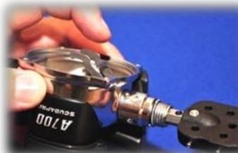
Continued! Lowering the lever (approximately a 1/4 inch) ensures, no interference when installing the inhalation diaphragm, resulting in a watertight seal. Tap the lever.
