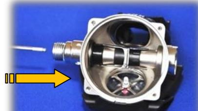
19. Push the poppet assembly free, using a blunt small diameter tool, like a 3/32 ball-end Allen driver.
