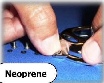
35. Press the screws, one by one, through the front cover hole and through the new 363 o-rings. The neoprene provides just enough support and give, to allow the screw to pass through the o-ring until installed.
