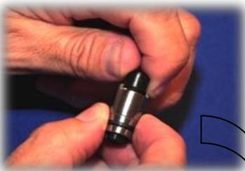
20. Screw the adjustment shaft into the metal sleeve.
