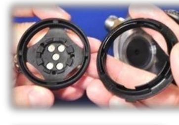
4. Separate the purge cover and ring. Inspect the integrity of the purge and ring. The metal, stainless steel "S" insignia is **not** removable.
