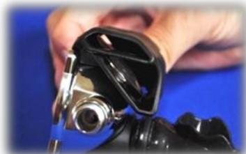
Note: It may be helpful to heat the exhaust T, warming a bowl of hot water in the micro wave or using a hair dryer.
