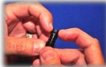
16. Spread the 351 o-ring onto the metal sleeve.
