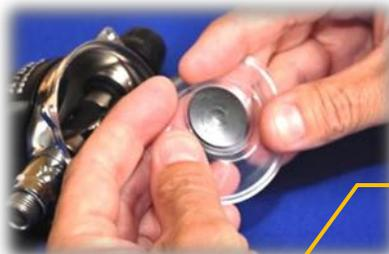
7. Inspect the smooth operating side of the disc for signs of wear. Replace as necessary.
