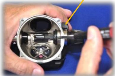
8. Next, remove the "dive switch" assembly. First remove the safety "C" clip by placing a flat blade screw driver in the negative detent (or the bottom side of the wave) of the "C"-clip.
