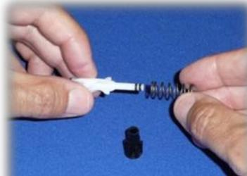
21. Remove balance chamber and spring.
