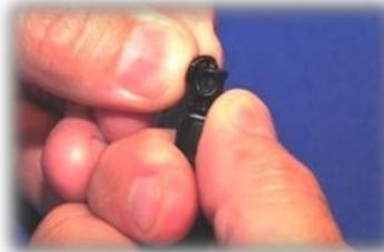
Once the 126 o-ring is in place, unscrew the “micro-adjust” and proceed.
