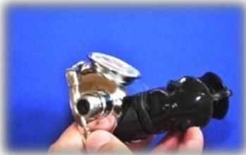
33. Look from the side to be sure the exhaust valve is laying flat and maintaining a good seal to the case.
