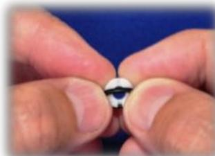
6. With the adjustable orifice slots at the 12 and 6 o'clock position – install the 132 o-ring using both thumbs.
