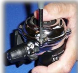
37. Begin to lightly snug the 4 TORX® screws down, using an X tightening pattern.
