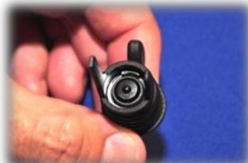
Note: Orient the metal sleeve tabs "north & south" in relation to the 2 (long/short) dive switch guides. The metal sleeve tabs engage into the case inlet-tube guides.
