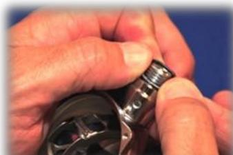
28. Lubricate and install the 347 inlet tube o-ring.
