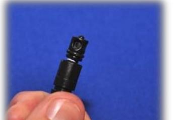
15. Following is *dynamic* application, lubricate the o-ring groove and slide the 293 o-ring down the “adjustment shaft, into the first/true o-ring groove. Then lubricate the male threads.
