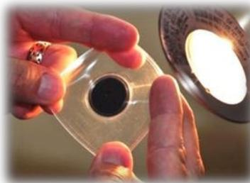
6. Hold the diaphragm to light and stretch it from 4 points to check for punctures. Reposition and repeat to be sure there are no punctures and that the diaphragm is imperfection free.
