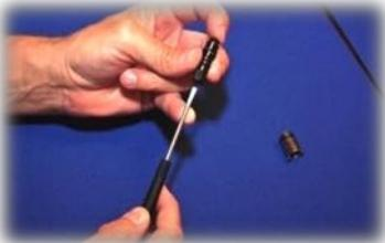
18. Using a flat blade screw driver, inserted through the shaft, turn the micro adjust *counterclockwise* until the micro adjust bottoms out.
