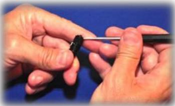
19. Preset micro-adjust as pictured below. That is, bottom out counterclockwise, and then advance clockwise exactly 2 full rotations – leaving a 1 mm step
