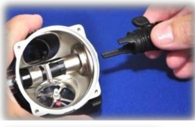
10. Pull the complete "dive switch" assembly free from the 2<sup>nd</sup>. stage case and remove the 2 o-rings, using a brass pick.
