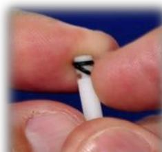
9. Pull the second o-ring onto the stem and use your nail to pull passed the first and into the (inside) groove.
