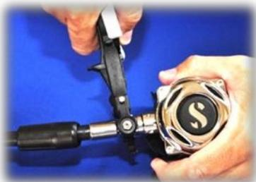
1. Pull second stage hose sleeve back – to expose LP hose swivel, loosen the swivel using the SCUBAPRO universal tool.
