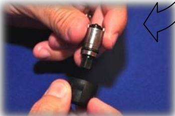
21. It is helpful to temporarily use the adjustment knob to finish – screw until the shaft bottoms out.
