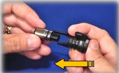
15. Screw the adjustment shaft clockwise, to separate it from the metal sleeve. In some cases, you may find it helpful to use the adjustment knob.
