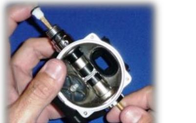
28. Expel the adjustable orifice with care, by pushing slowly from the “knob” side of the inlet tube. Your tool of choice must clear the lever tabs and orifice knife-edge.
