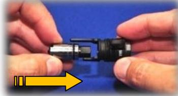
23. Push the adjustment shaft sub-assembly into the "dive switch".
