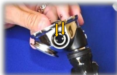
26. Look inside the inlet tube, with proper lighting – to be sure both lever **tabs** (deep inside the inlet tube) are present and imperfection free.
