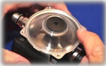
31. Be certain the entire circumference of the diaphragm is laying flat and into the case diaphragm groove.
