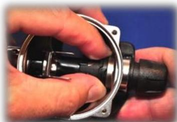
27. Press the clip "top & bottom", to be sure the new clip is correctly engaged.
