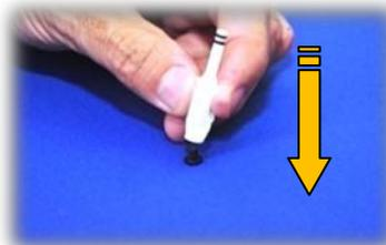
10. Utilizing a clean hard-flat surface – firmly **press** the poppet onto the LP seat, uniformly.
