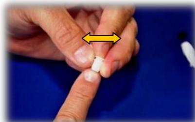
30. Now thoroughly inspect the knife-edge surface using your finger-nail to detect any nicks or imperfections, by rotating the orifice back and forth.
