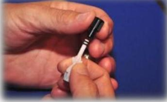
11-A. **Seal** the LP seat hole with thumb.
