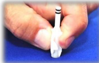
Note: Wipe the surface of the newly installed LP seat, to remove manufacturing residues.
