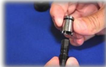
16. Remove both the shaft o-ring and sleeve o-ring, using a brass pick.
