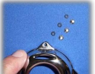
34. Align one cover hole with an o-ring.
