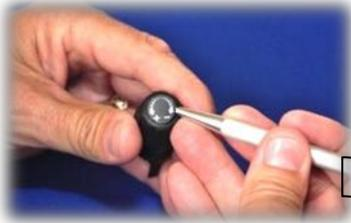
11. Lift the decal from the adjustment knob, using a suitable device. A new decal is supplied in the A700 maintenance kit.
