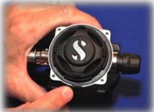
33. Place the two piece assembly, orienting the ring tab into case notch located at the "6 o'clock position".
