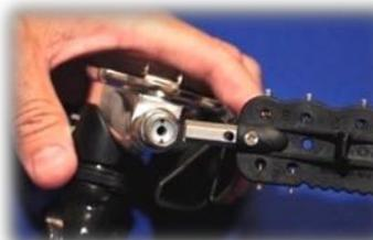
29. Engage function #7 into the orifice slots. Screw clockwise until the lever drops slightly.
