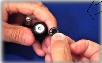
12. Unscrew the 4 mm adjustment knob Allen-screw and remove the o-ring.
