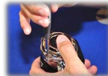
2. Using a TORX® T10 driver, remove the 4 front cover screws.
