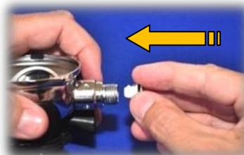
7. Apply a dot of quality lubricant to the beginning threads. This will ensure easier removal during the next service. **Simply push orifice into inlet tube. No adjustment yet!**
