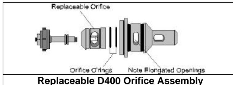
Because of the re-design of the orifice, the brass poppet housing is also of a different design. All D400 configurations fit into older and more recent regulator bodies, but a complete replacement of the brass poppet housing must be made in order to take advantage of this snap-in orifice improvement.
